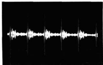
SSB Signal Before Processing. The weak valleys and high peaks give a low average power output, resulting in a real lack of punch.
