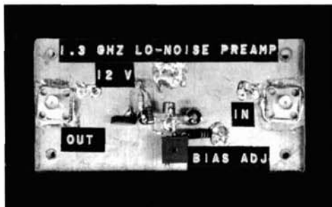
Ground-plane side of the preamplifier stage. Note that component placement in the dc bias circuitry is not critical but the feed-through capacitors make convenient stand-offs. The transistor mounting hole is covered with copper foil to promote good rf shielding.
