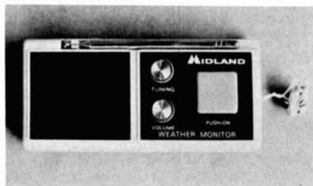
This particular model receiver already had a very small trimmer "Tuning" control to provide reception of either 162.40 MHz or 162.55 MHz.
