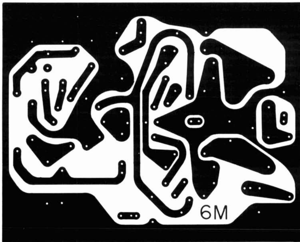
fig. 3. Full-size printed-circuit board for the transmitting mixer.
