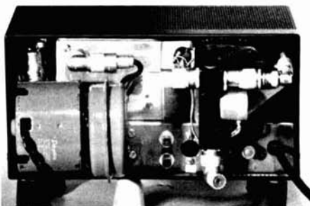
Rear view of TR-50 shows blower and Dow-Key antenna changeover relay.
