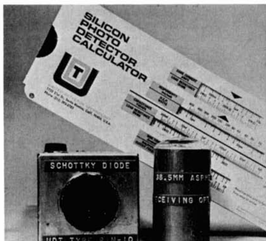
The UDT type PIN-10 broad-area detector, recommended for laser diode receivers. The receiving optics were discarded, because surface pickup is important rather than narrow-beam optical gain with these detectors.
