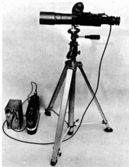
The M3 Sniperscope, battery, and high-voltage power supply. Unit is essential for collimating laser energy and boresighting.
