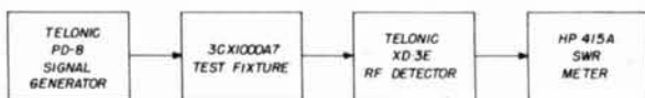
fig. 3. Block diagram of the test setup to determine the self-neutralizing frequency of the 3CX1000A7 triode and SK870 socket.
