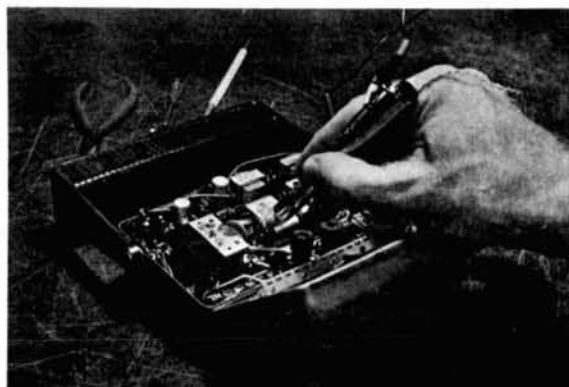
fig. 1. Servicing a small two-band portable radio with a pencil-type signal tracer.
