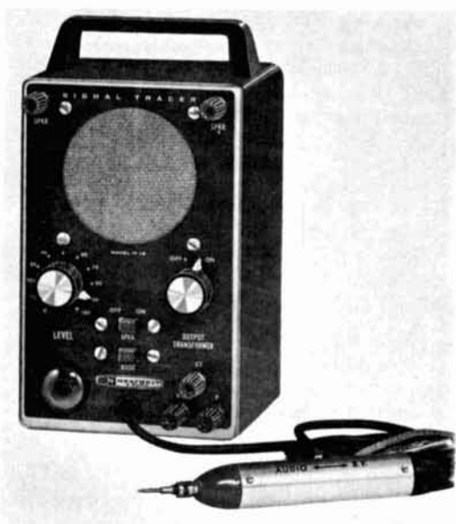
Kit-model signal tracer is high-gain (and quiet) audio amplifier. Probe can be used direct or with switch set for demodulation.
