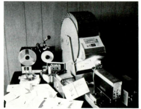
The entire package of TeleShop'r equipment takes up a space 14" wide by 40" long and 27" high.
