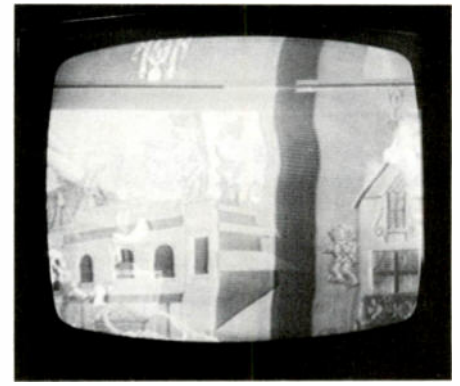
The left photo shows a TV screen with no interference. The center photo shows the same scene with beat pattern resulting from direct pick-up. At the right is a phase-locked operation with one station superimposed over the other. Due to phase-locking, there is no interference beat. This is an extreme pick-up case.
