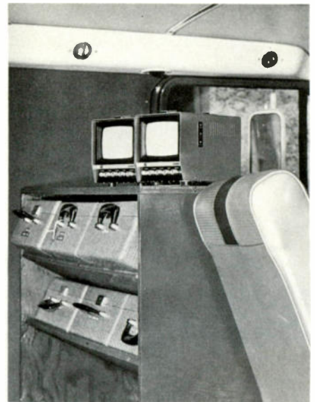
Other side of panel truck interior holds two GBC 5" monitors and cases containing cables, intercom headsets and other accessories.
