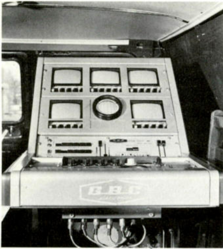
Inside panel truck is GBC control console, with 5 monitors, switcher-fader/special effects generator, audio mixer, sync generator, intercom and tally lights.
