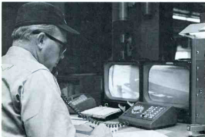
Closed circuit television system helps in security and surveillance at jet freight terminal. Two cameras outside the building, and two inside, sweep the area giving air freight coordinator, shown watching dual monitors, picture of the entire facility. Television system also helps coordinate sorting and processing of freight.
