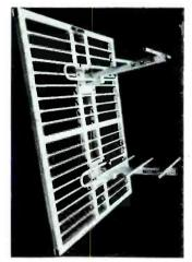
Multiple ruggedized yagi array mounted on screen reflector for maximum front-to-back ratio.
