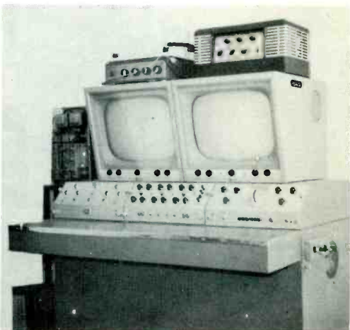
CONTROL CENTRAL at Oneonta Video, Miratel monitors and audio-video mixing board.
