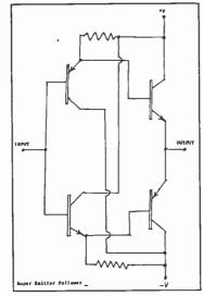
drive transistor cancel out the .7 of the output transistor so that the input bases can be tied together. See diagram. This circuit has the additional advantage of having a very high input impedance due to darlington connection. This allows DC restoration at the input with very little leakage. A driven clamp can work quite well clamping to the back porch.
