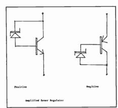
assuming you have chosen a transistor that can handle the power.
