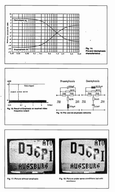
The form of the characteristics are shown in fig. 14. The networks are of a simple nature and are installed in the video frequency circuits of both transmitter and receiver.
