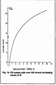
At a modulation index of M = 1, the bandwidth is about 22 Mhz and the FM gain (over AM) is 6.7 dB. This should be a satisfactory working condition for the SHF bands. The satellite TV bands, however, use a somewhat larger bandwidth of 27 Mhz. At я modulation index of M =5 the bandwidth would be an enormous 66 Mhz at an FM gain of 20.6 dB. It is clear that gain is purchased at the expense of bandwidth in an FM
