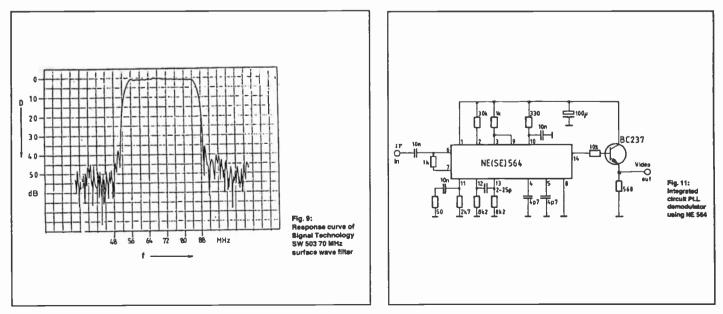
The pass band flanks are fairly steep in order that adjacent channel narrow band signals (CW, SSB, FM speech) do not interfere with the reception of FM ATV signals. A sweep generator is required for alignment. A pre-aligned, 70 Mhz mid-frequency LC bandpass filter is now available from Texscan with bandwidths of 16 to 30 Mhz (designated e.g. XBM 70/25-1). Its use obviates the requirement for a sweep generator.
