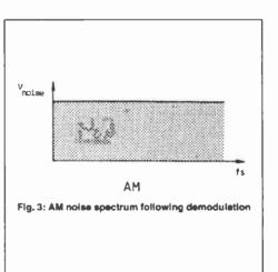
The noise spectrum located about a demodulated AM carrier, in the absence of distortion, is of constant amplitude (fig. 3) with frequency.
