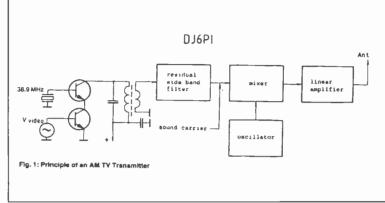
verter. The ATV signal is then translated into a suitable channel at VHF or UHF. As the picture information is contained in an AM signal, all stages in the transmitter must work in a highly linear mode. All departures from amplitude linearity have the effect of displacing the horizontal picture lines thus distorting the picture as well as falsifying the contrast and color content. The signal also suffers from reduced synchronization leading
