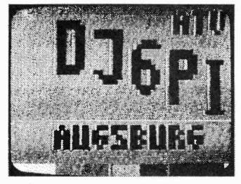
Fig. 25: As fig. 23, but Po = 70 W, C / N = 30 dB, slight noise, colour present
