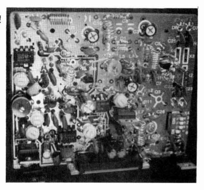
MODULE CAN BE PURCHASED AND SOLDERED IN LATER FOR 5 WATT AVERAGE OUTPUT POWER. POWER WITHOUT MODULE FROM DRIVER IS APPROXIMATELY 50 MILLIWATTS.
