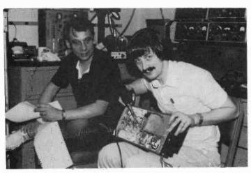
"Fit it!" Less than 24 hours before the scheduled uplink, the Motorola amp gave up. Gene W3PM and Larry WA4CAX switched transistors to get it working.
