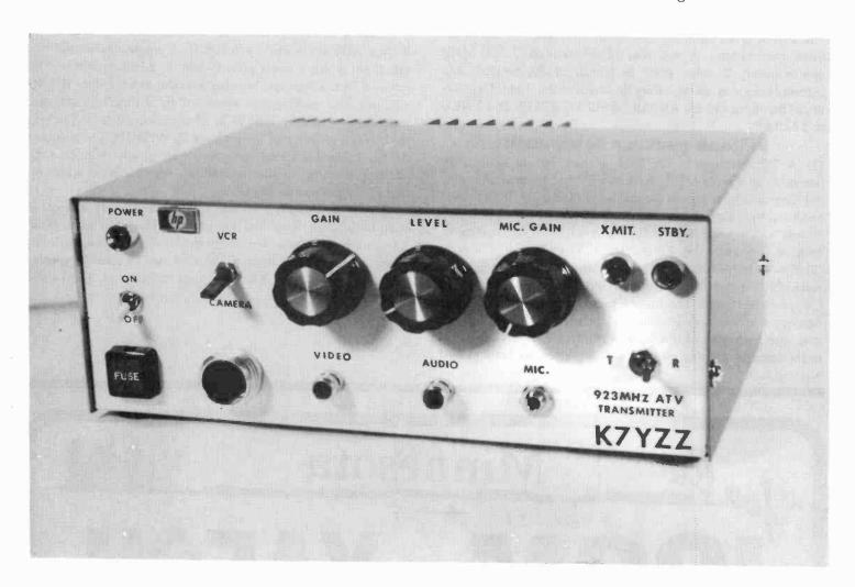
Two circuit boards were ordered from PC Electronics. The TXA5-33 1 watt ATV Transmitter and the FMA5-E Sound Subcarrier Generator. A 5 watt RF Power Amplifier "brick" was ordered from Pauldon Associates.
