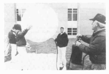
As another part of their experiment, they build two different radar reflectors out of metalized Mylar. They attached the smaller one to the flight line of the ATV balloon. In addition, they built a large reflector (garbage can sized) which they flew on a separate small balloon (no transmitters on this one). They hoped that the local Indianapolis Center FAA office could actually see the radar reflections and track the balloons.
