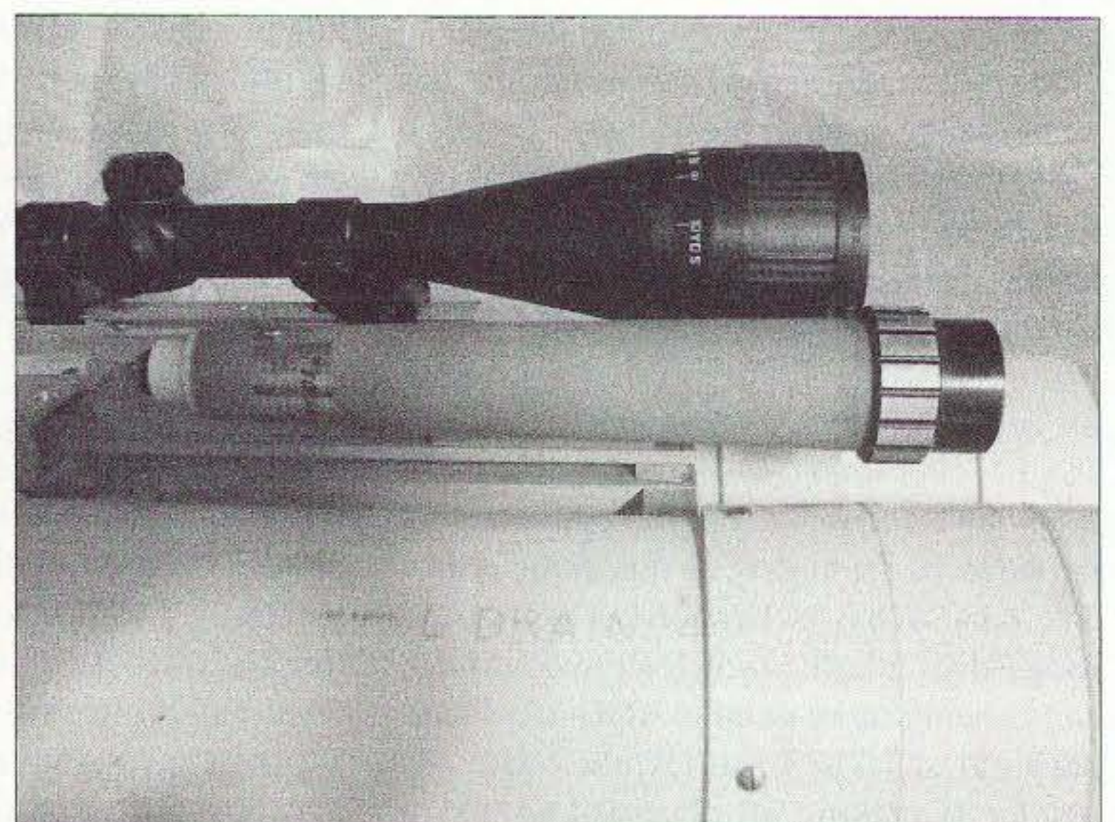
Photo B. Picture of another beam expander using old objective portion of spotting scope with the laser and first lens in PVC pipe at far left showing diversity in construction that also works well. It's the optics, not the construction methods.
