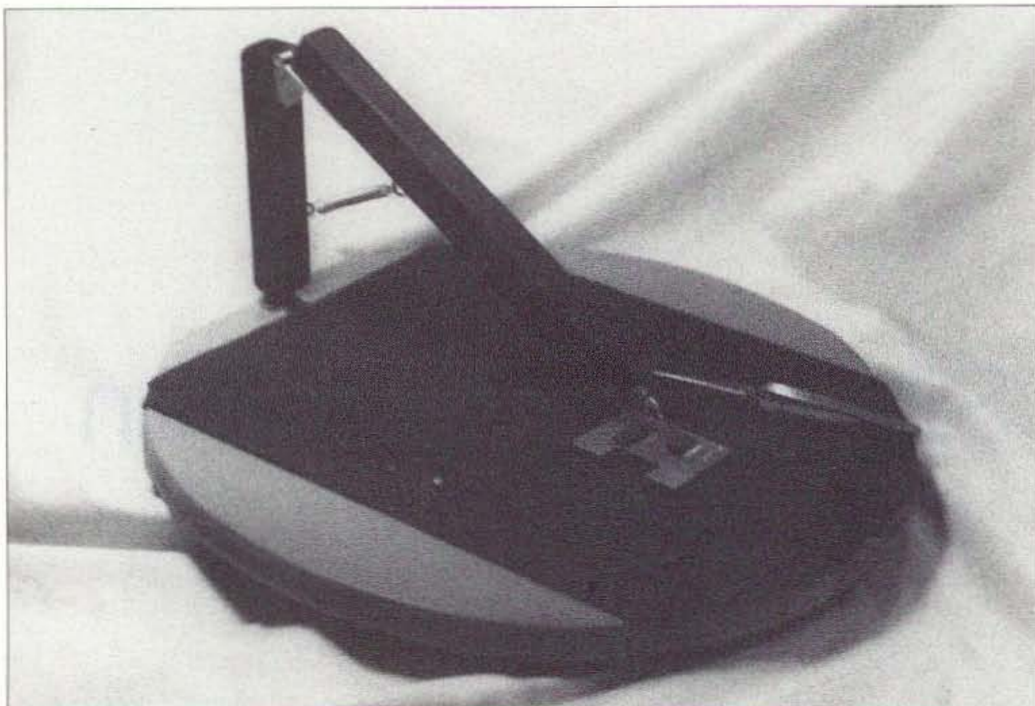
Photo A. The completed SMT work station, ready for operation. Not high-tech or difficult to build, it does make assembling a surface mount project much easier to do.
