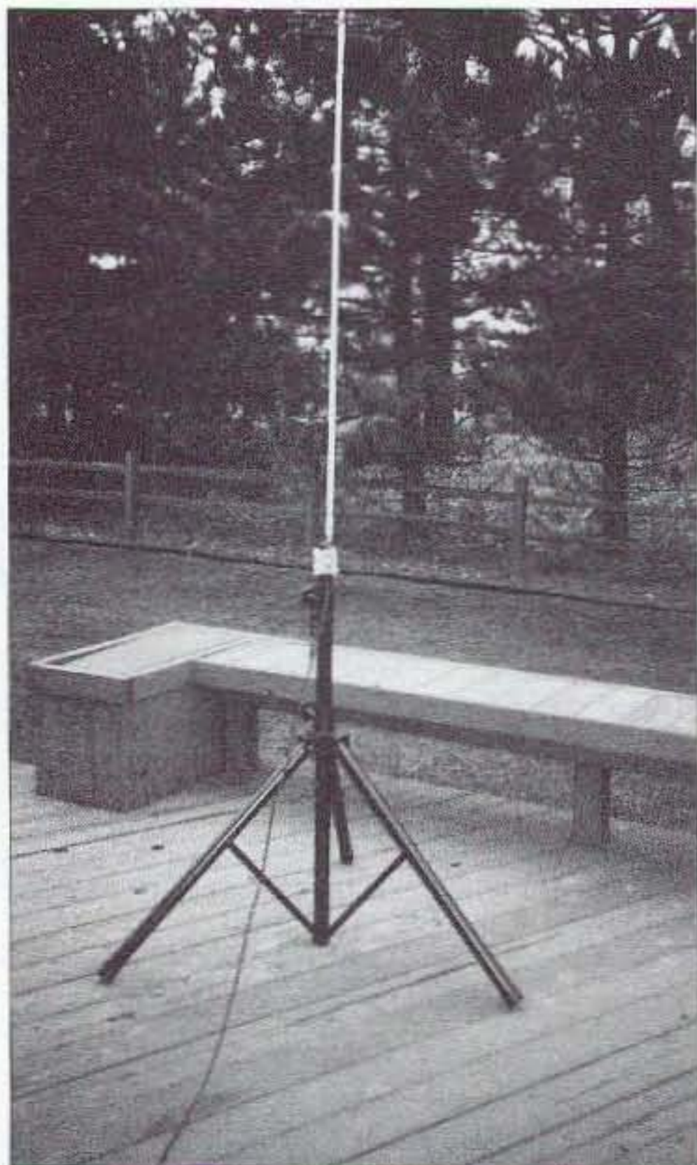
Photo A. The Cheap & Easy Portable HF Vertical securely mounted on a speaker stand.
