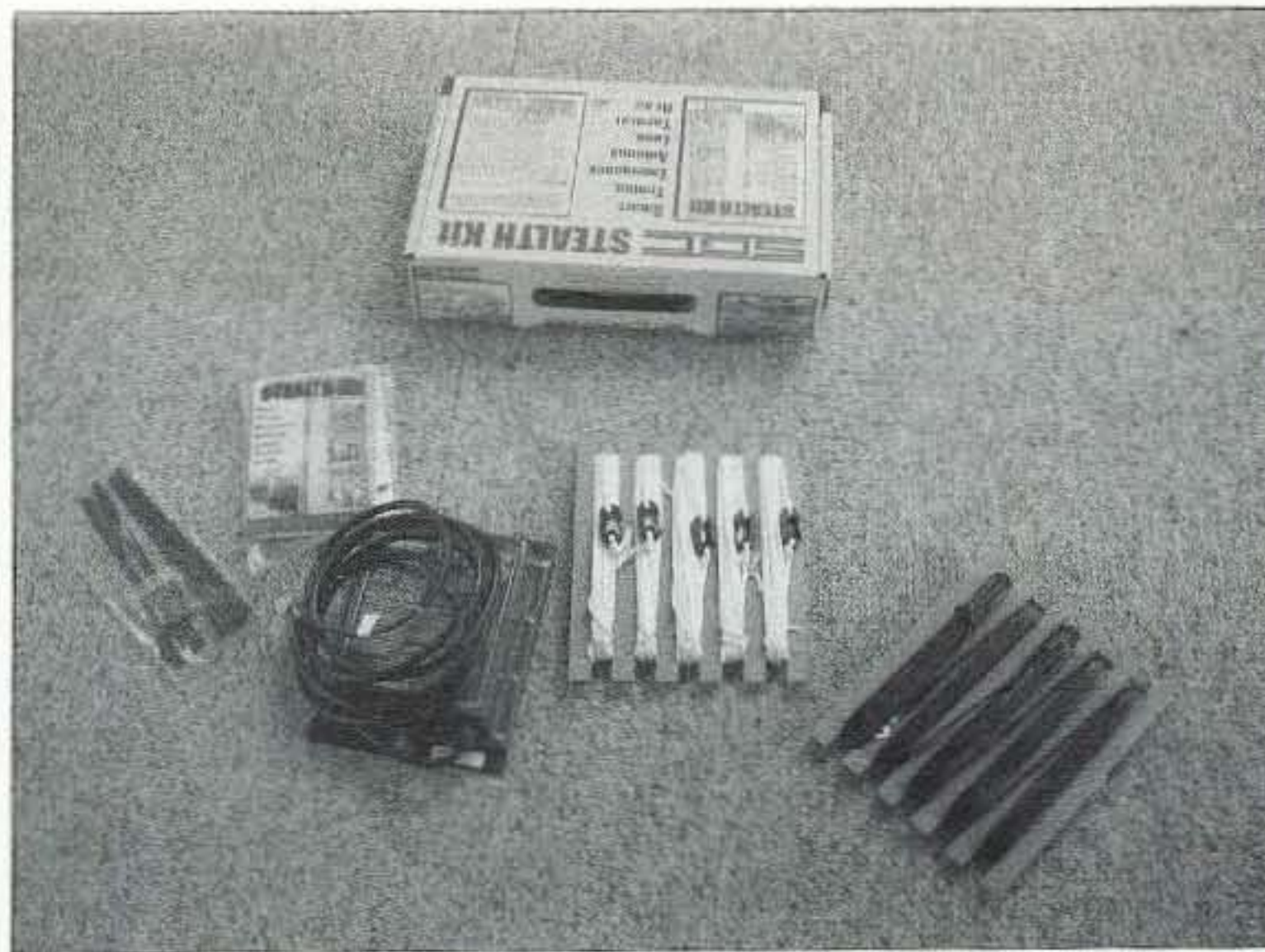
Photo B. The kit contains 80 feet of wire, nylon lines with insulated clips, reusable cable ties, the Smartuner, and manuals. Add a radio and 13.8 volts DC, and you're on the air.
