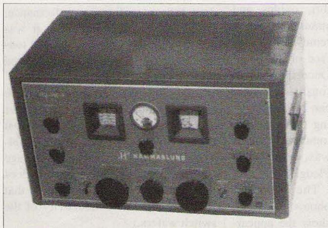
Photo A. The receiver as it was removed from storage. Note the dirt on the cover and the dark stains around the knobs.
