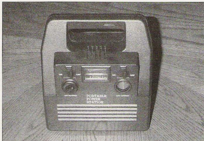
Photo A. The Power Station 2 includes a durable case, two cigarette lighter outlets, and a voltage meter. Weighing about seven pounds, it can extend your operating time.
