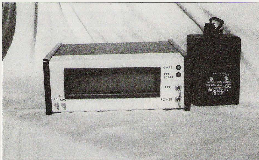
Photo A. The K8IHQ high-performance frequency counter.
