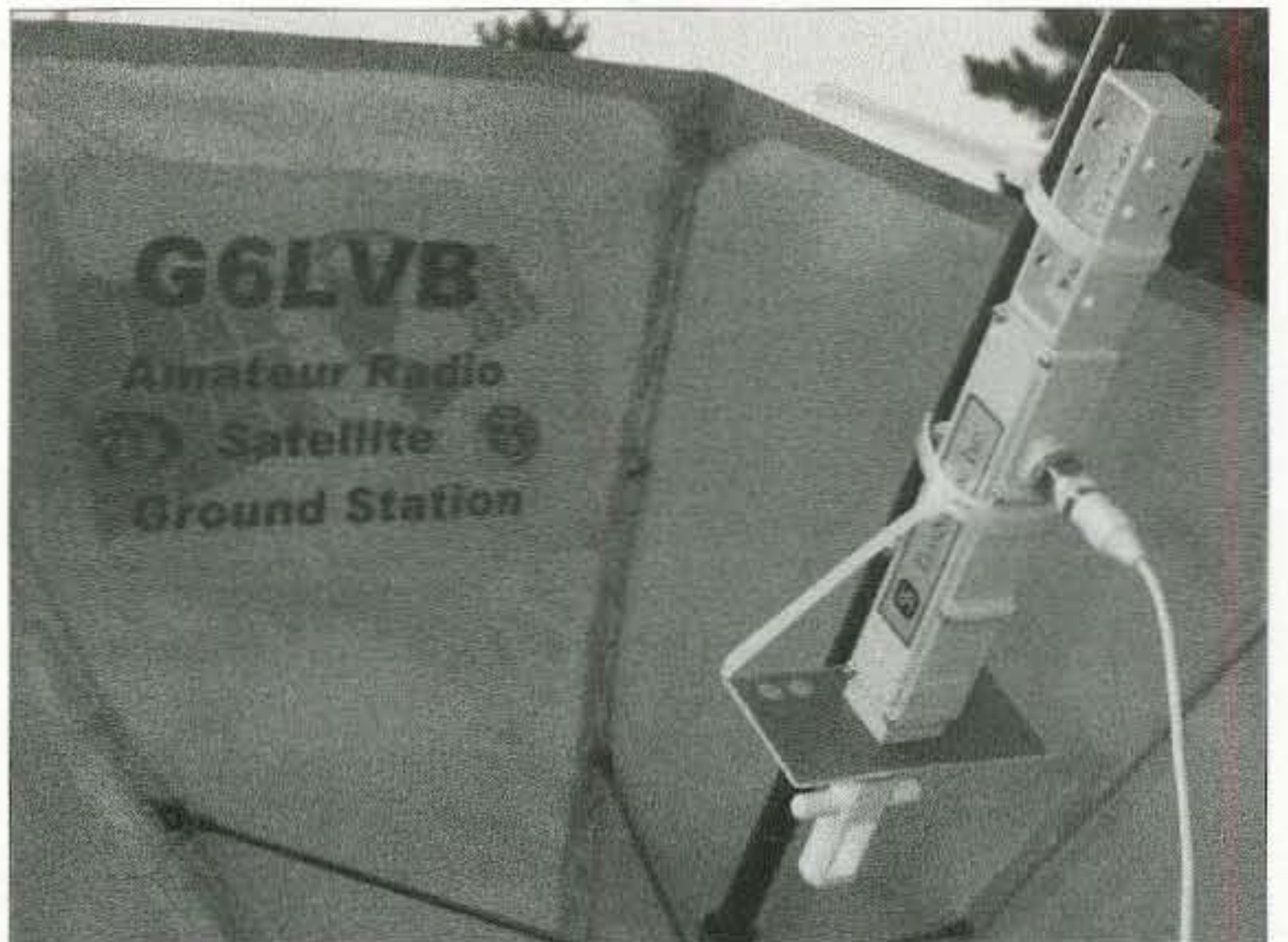
Photo D. A close-up of one of Howard G6LVB's 2.4 GHz downconverters positioned in front of his Umbrellantenna. What was an umbrella is now a dish antenna covered with metal fabric.
