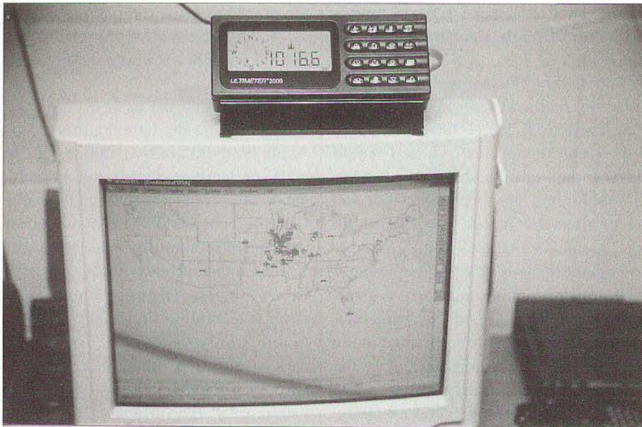
Photo E. The "brains" of the Peet Brothers Ultimeter 2000, showing display of the data and the control panel. The unit is connected to the computer below and from there to the TNC and 2-meter rig for APRS operation.
