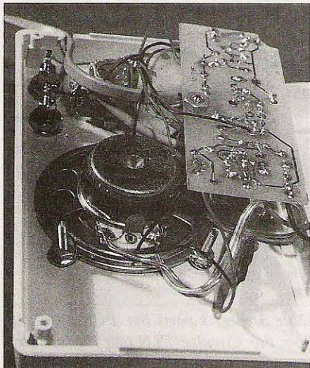
Photo D. Interior view of model B ( Photo B ). AUX INPUT upper left of photo. Notch in box for input connector with RJ11 plug. Volume control and ON/OFF switch, top center. Notch in circuit board allows it to fit in this box, which has a special compartment for a 9 V battery.
