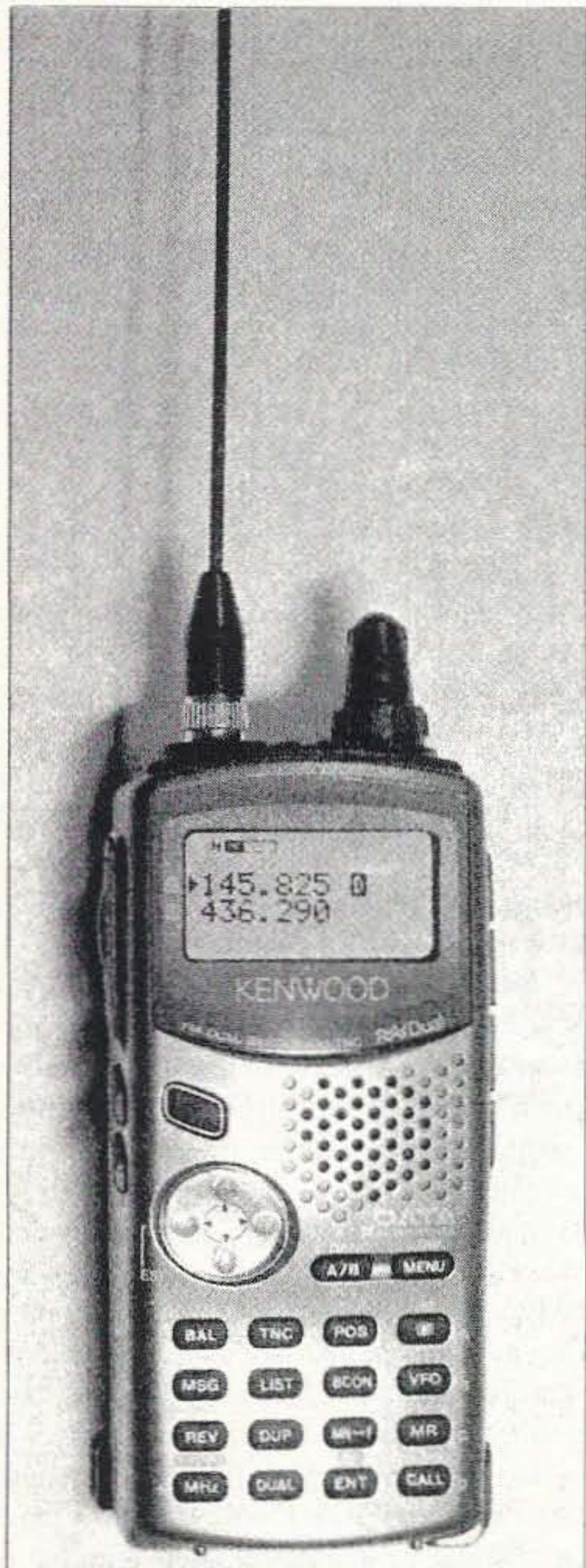
Photo A. The Kenwood TH-D7 HT has built-in 1200 and 9600-baud packet with APRS support. A long dual-band antenna makes it useful for pacsat work or crossband voice operation.
