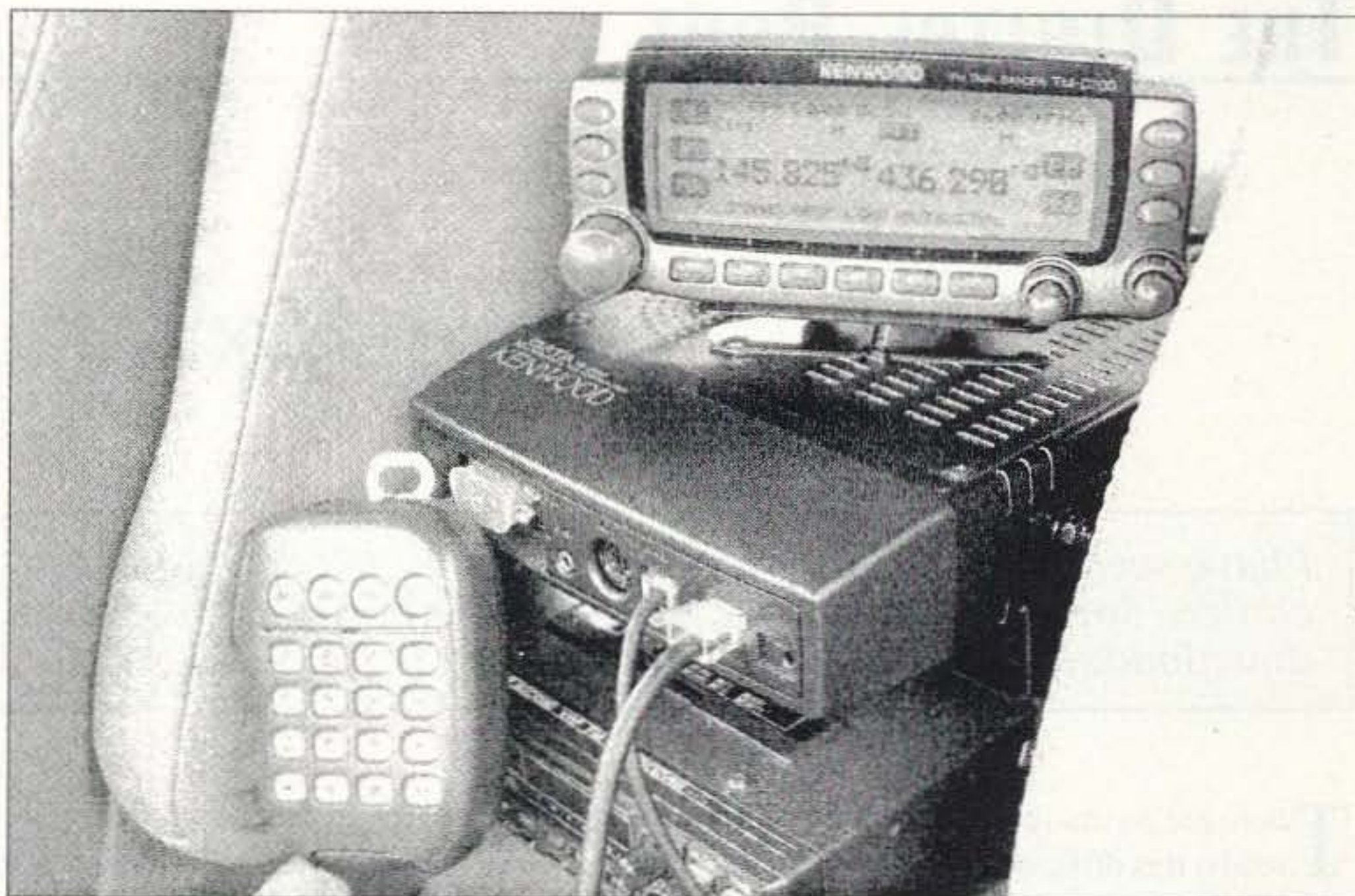
Photo B. The Kenwood TM-D700 mobile radio can do stand-alone APRS transmission and reception from hamsats that support digipeat operation in addition to other pacsat and voice-satellite activity.
