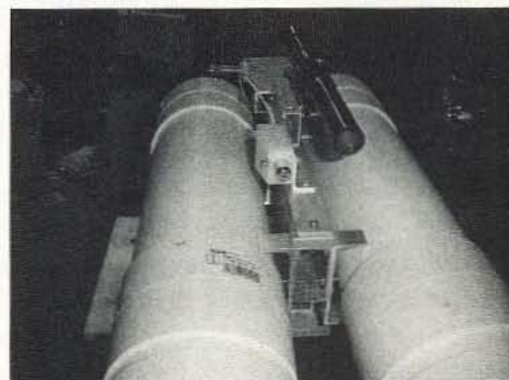
Photo C. Photo of the rifle scope mounting on top of the main rectangular support. The "L" bracket for the scope mounting is slotted on the rear end of the main mount for vertical movement to align to scope to the LED light source. The bottom of the mount rear is slotted for horizontal alignment of the same scope.
