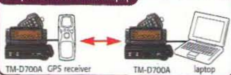
Example A: with GPS receiver & laptop
