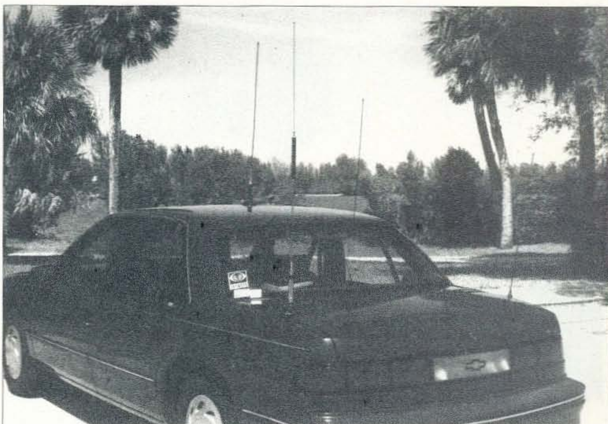
Photo A. Before — Here's my car with a twenty-meter antenna on the trunk lid, two-meter/seventy-centimeter glass mount antenna and ten-meter magnetic mount on the roof. I've been accused of having a car that looks like a porcupine.
