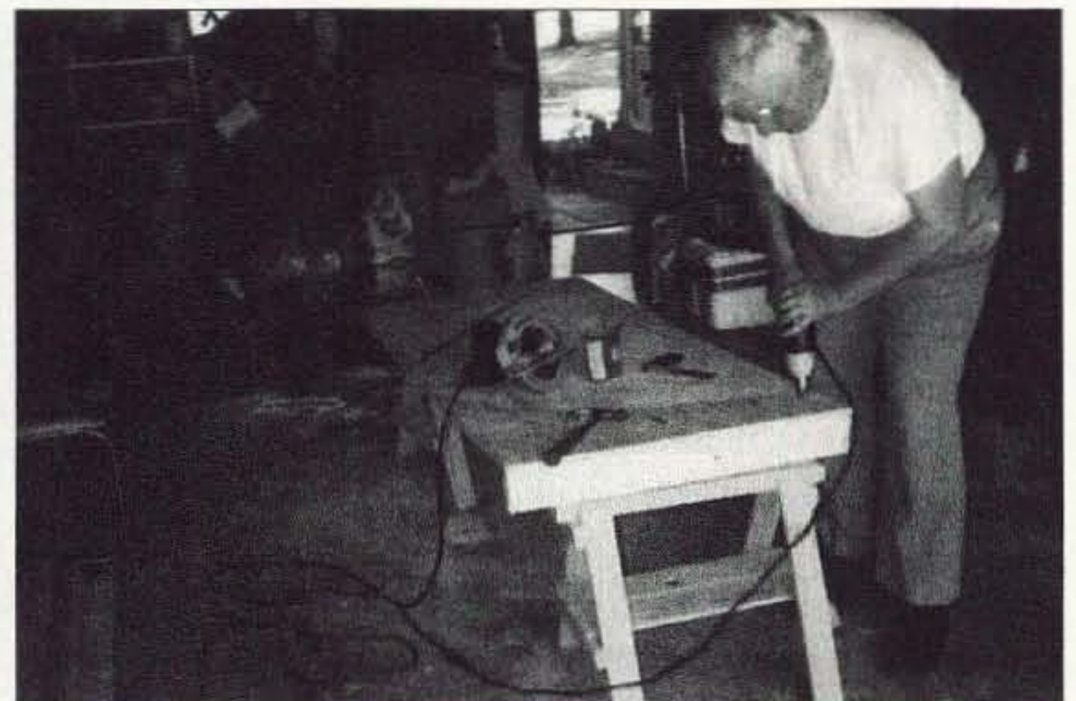
Photo B. You can use a nail tightly set in your drill chuck to make nail holes ...
