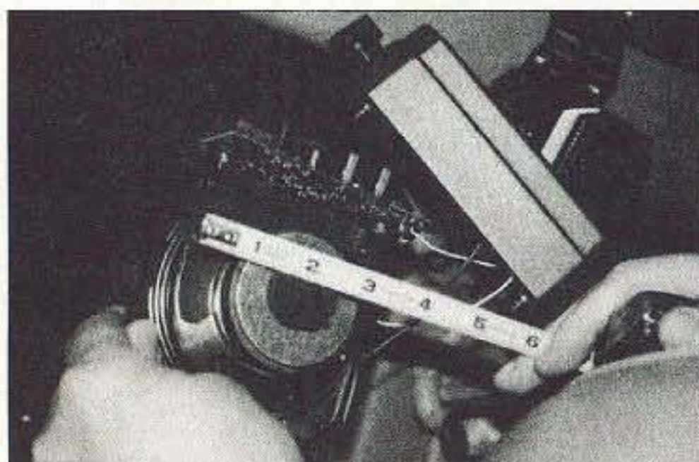
Photo D. Large speaker moves a lot of air but adds to the heft of the ClearSpeech unit.
