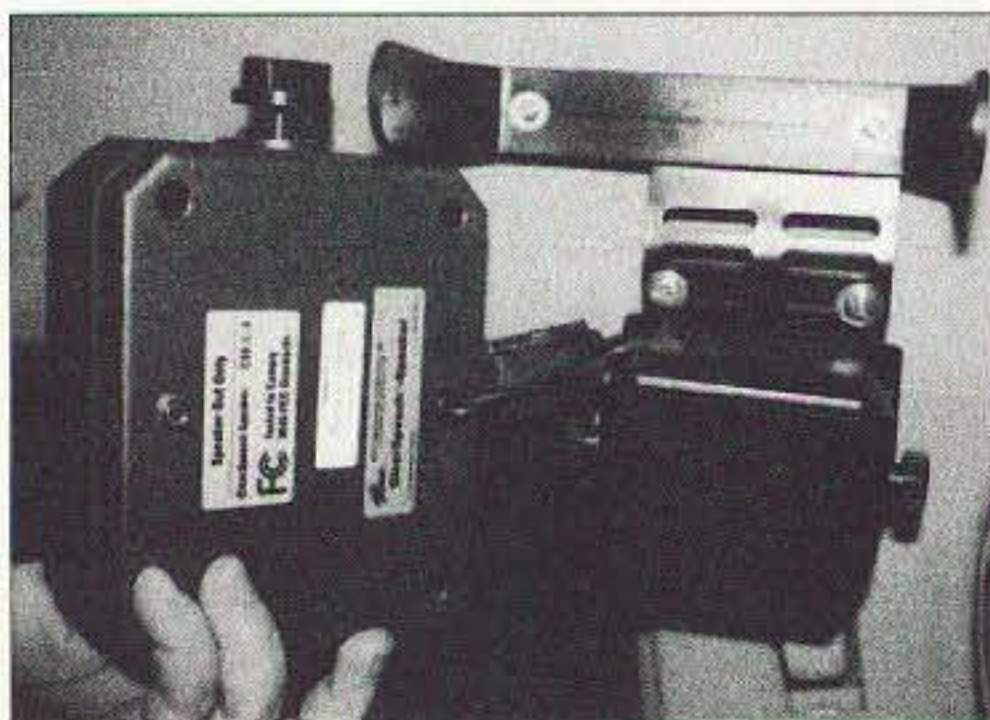
Photo C. Audio and power leads to ClearSpeech are mounted low on its case. Toroid is mounted on power leads outside case and is depicted as shipped from the factory. Note "Auxiliary Speaker" jack at top of ClearSpeech case.
