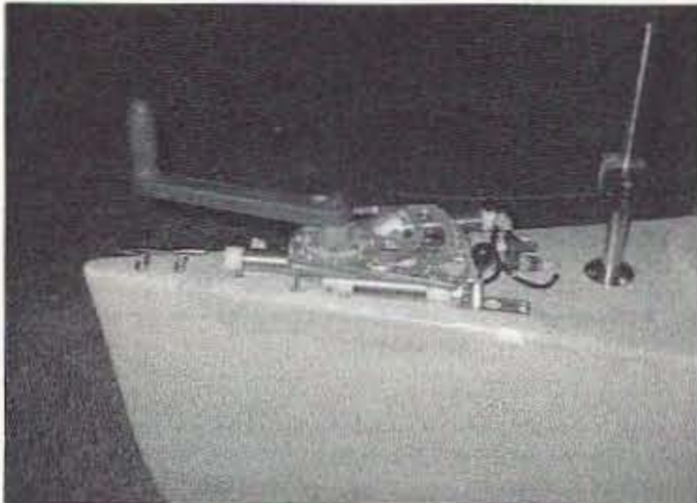
Photo C. Hydraulic controls for landing gear steering, using a cam follower to implement the Ackerman function and a separate control arm to "pigeon toe" the front wheels for hill-holding — a sort of software brake.
