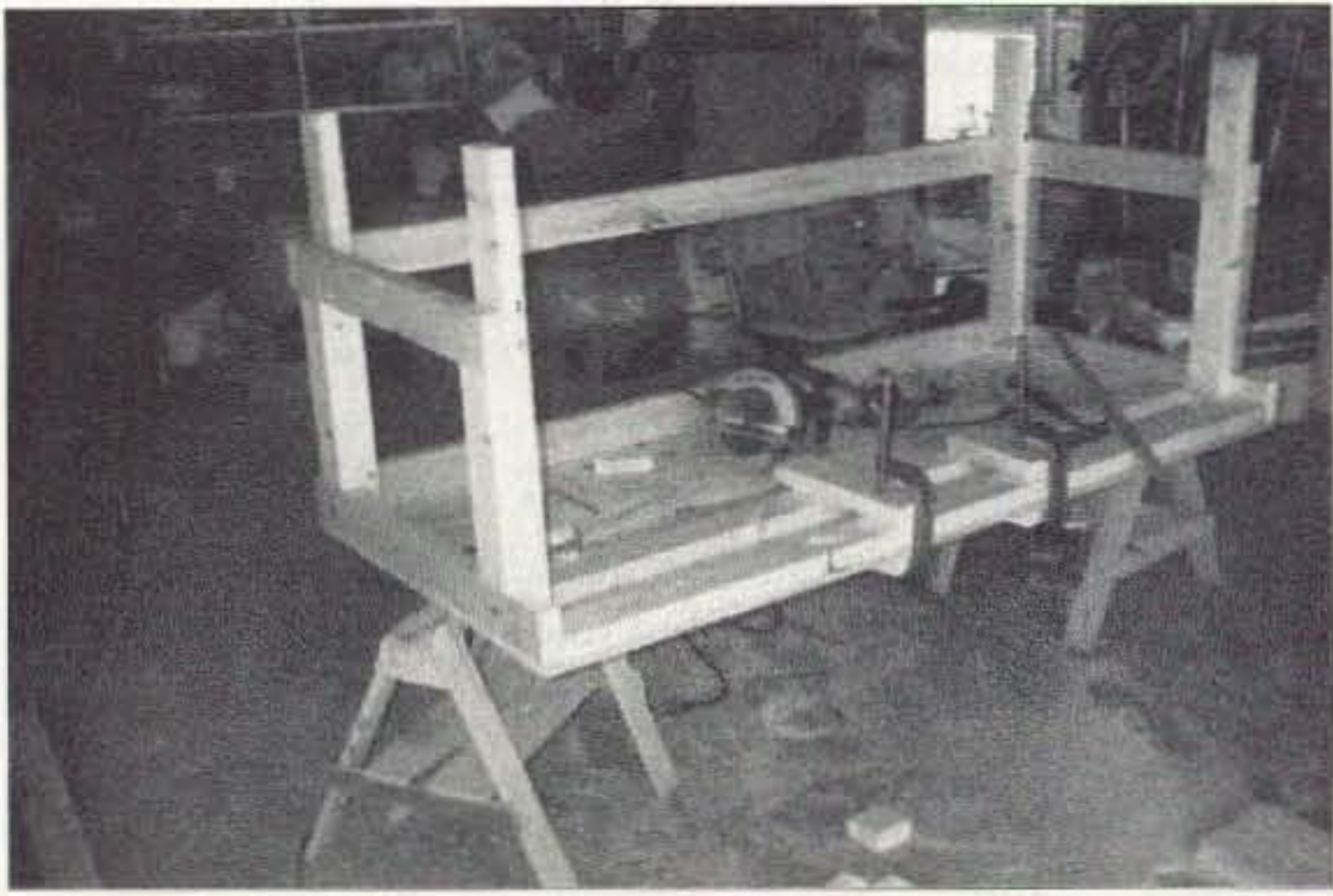
Photo G. Cut two pieces equal to the overall length of the table ...
