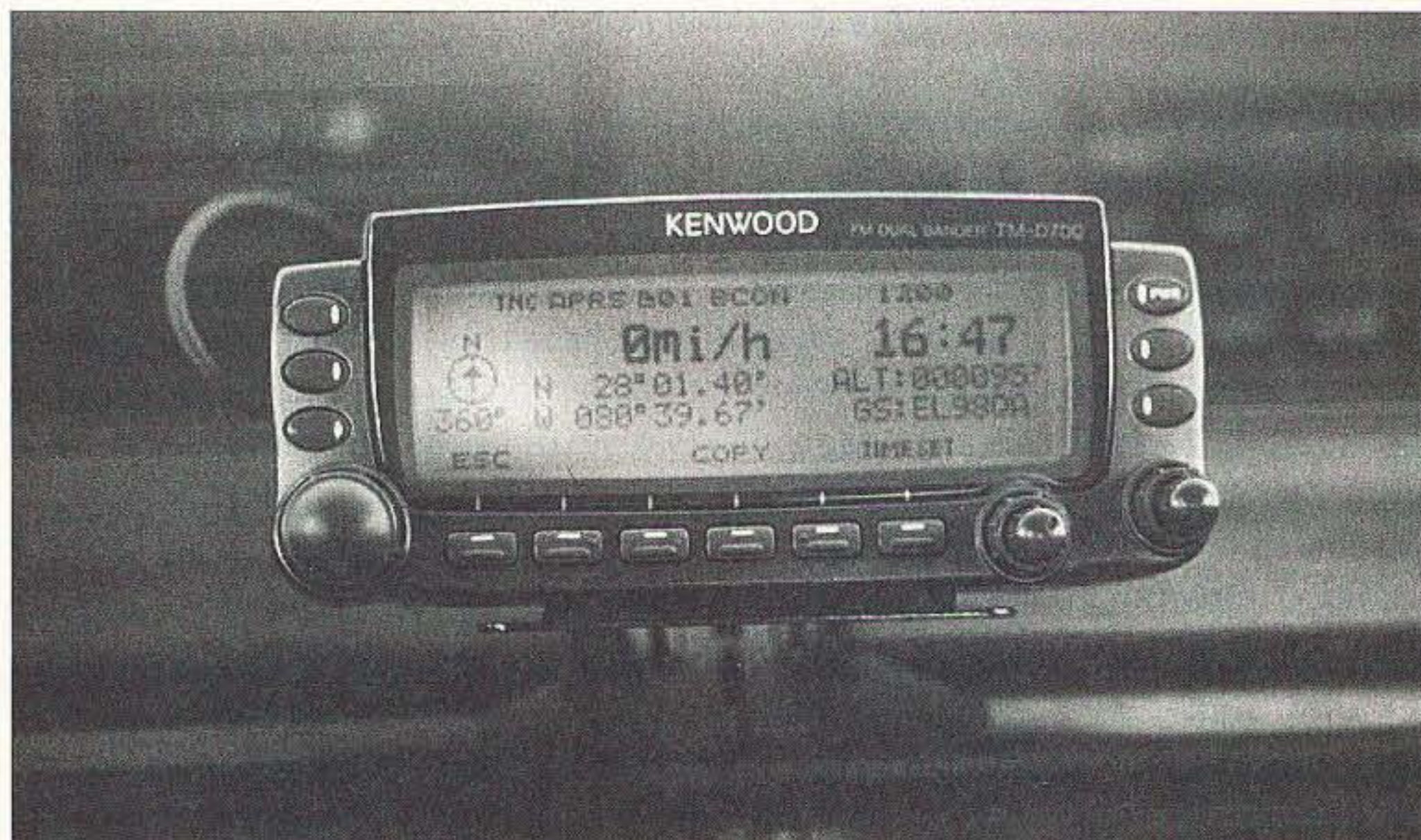
Photo C. If you have a GPS receiver hooked to your Kenwood TM-D700A, the control panel can show key data including speed, heading, latitude and longitude, and even the current grid square.
