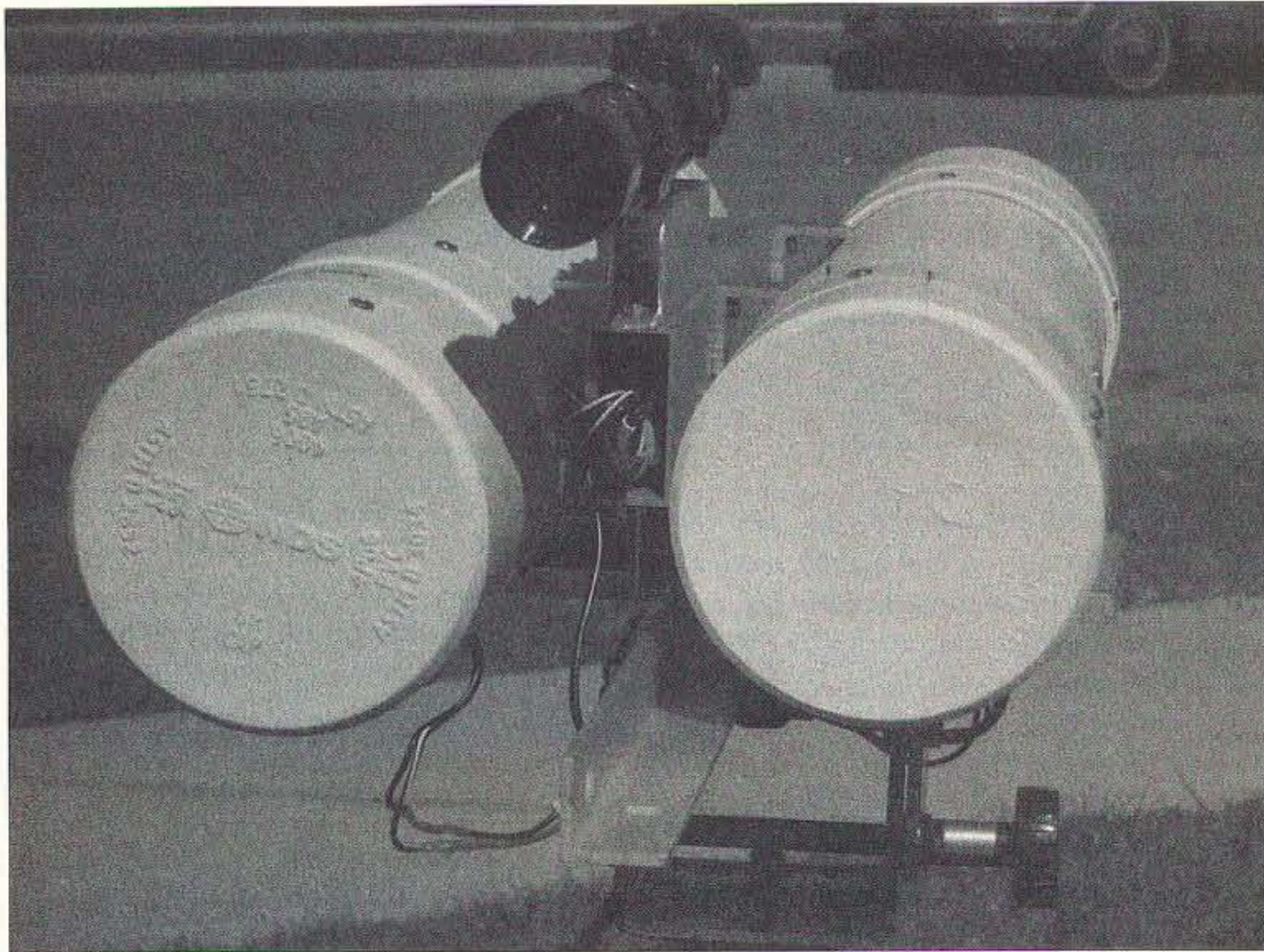
Photo B. Rear photo of LED transceiver with pipe caps in place on rear of system. More detail of aluminum rectangular tubing and "U" brackets to side of main support for "U" bracket holding 4-inch pipes in place. Additional rectangular aluminum tube attaches rifle scope on top of main support aluminum. All mounted on heavy plate for tripod mounting.
