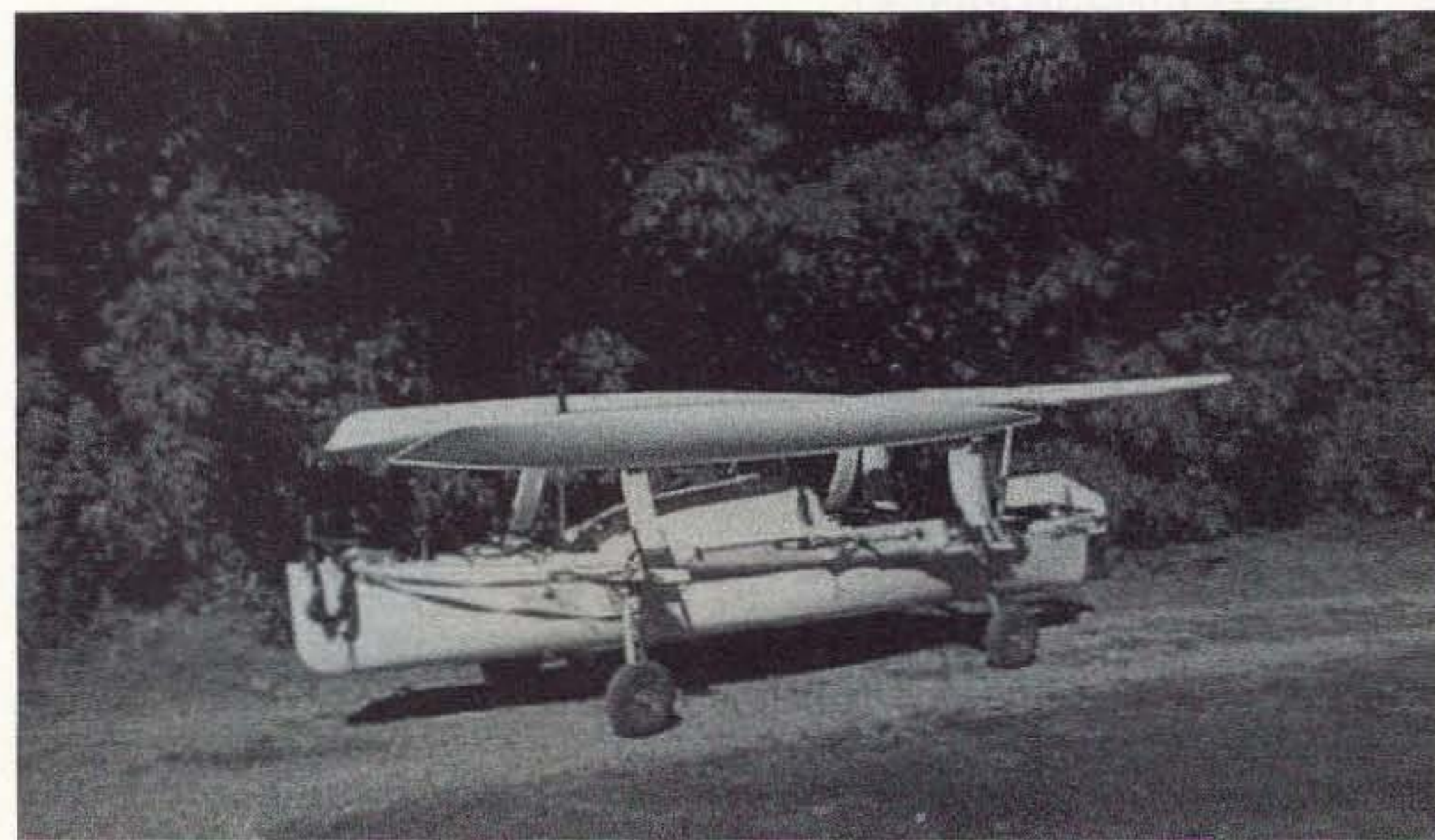
Photo G. In "land mode," deployable landing gear allow easy portaging, though hills can be challenging. We haven't figured out what to do about gravity yet.
