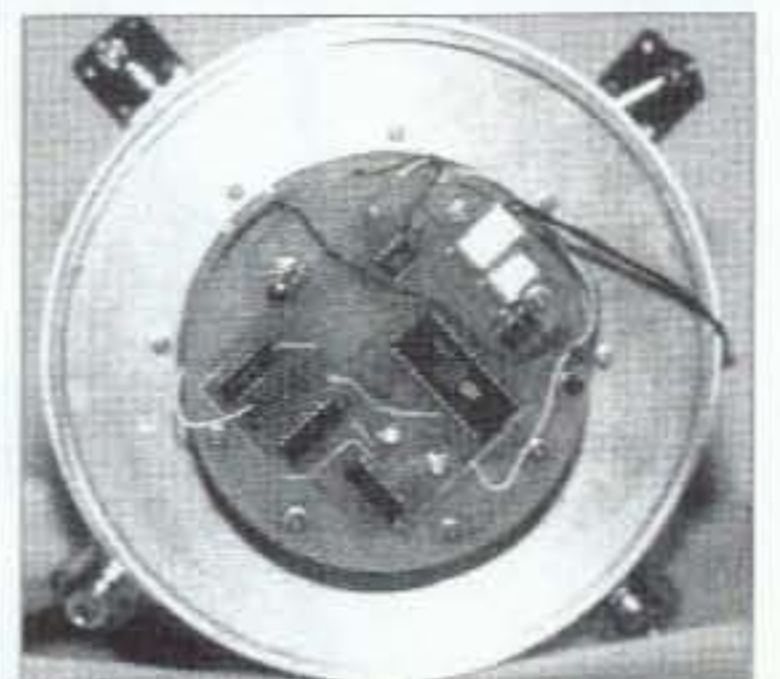
Photo C. View of the voice module on RS-18 includes a 90-second memory chip and supporting circuitry.
