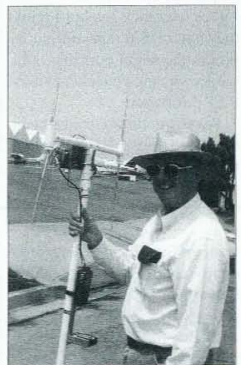
Photo B. Bob Legg W6QYY has his dual-antenna TDOA set ready for "sniffing" duty at the Montgomery Field starting point near San Diego.
