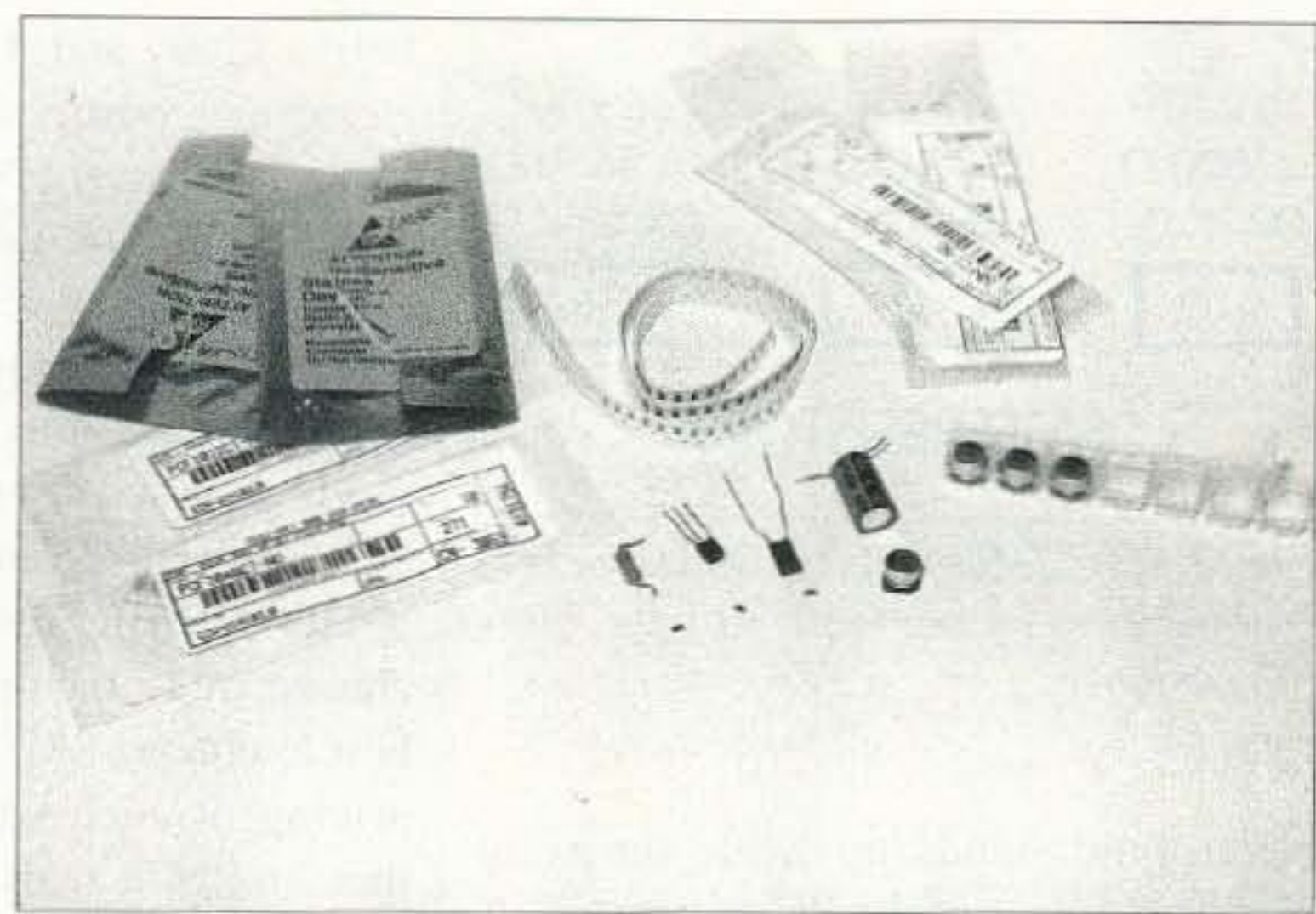
Photo C. Four tiny SMD chips are dwarfed by their common equivalents. From left: resistor, transistor, fixed cap, electrolytic.
