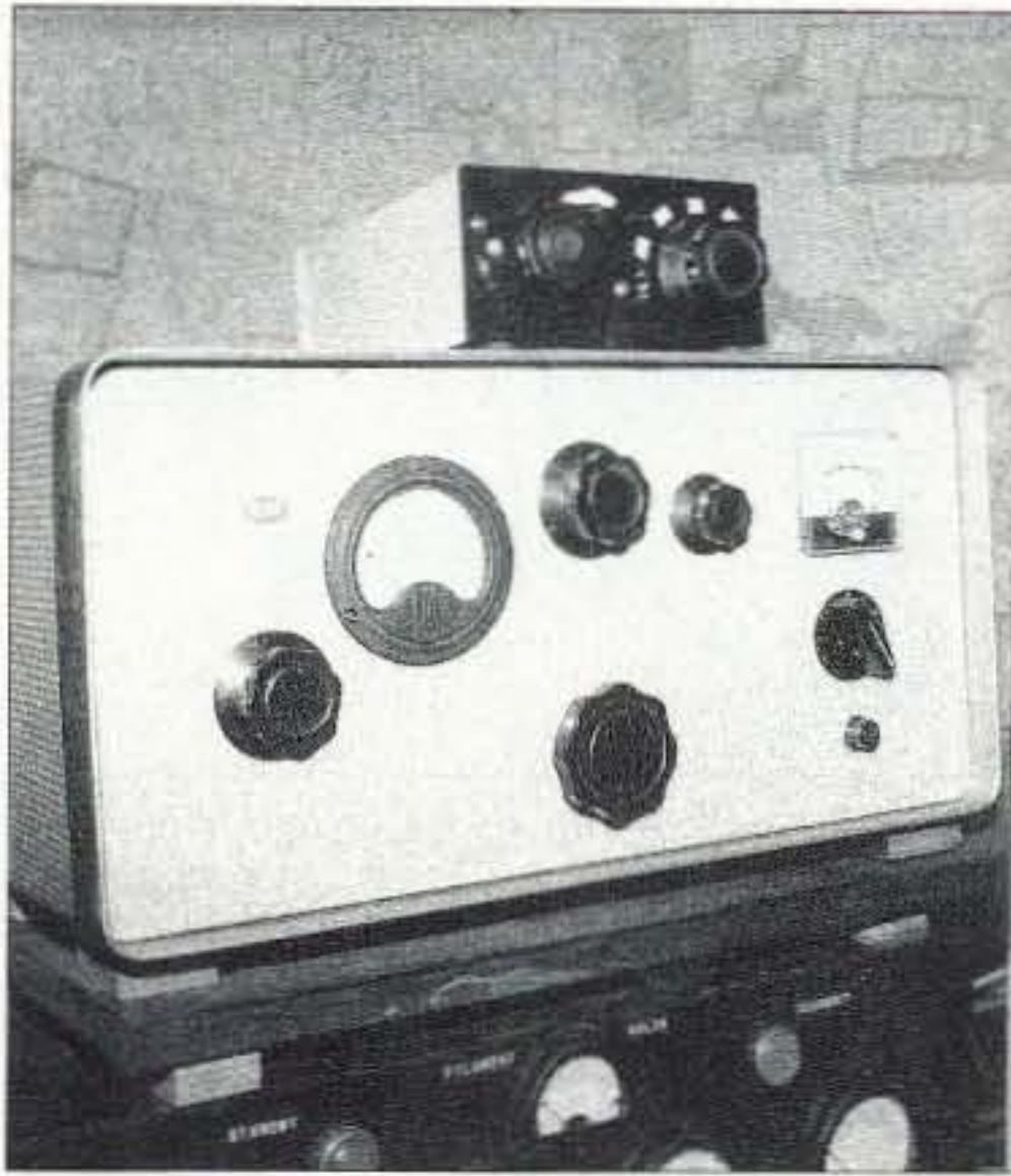
Photo A. A view of the tuned input module resting comfortably atop a three-hole 813 B&W LPA-1 amplifier deck cranking out 1000 + watts into the antenna. Output has been substantially improved with the input module installed. All photos by author.
