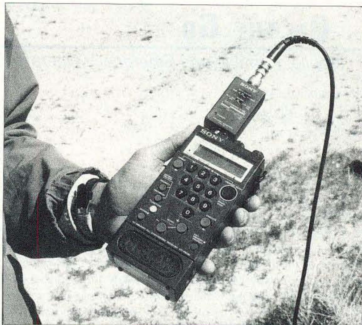
Photo B. This researcher uses a Sony multimode receiver and attenuator to track pulsed signals from tags on desert tortoises in California.
