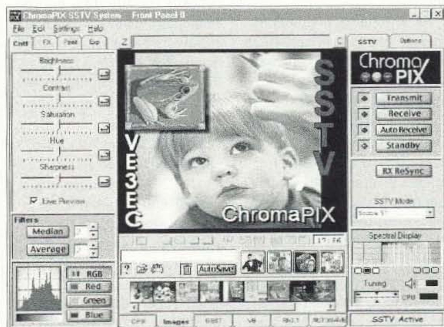
Fig. 1. Scanned from the manual, this is what the program looks like on your monitor. At lower right are tuning aids. Above those are the mode choice menu, and then the transmit and receive buttons. At middle bottom is file handling, and to the left are controls for editing the image. Clicking tabs gives access to more features, including received image filtering and more editing choices. I tried a live screen save to the clipboard, but the quality was very poor, so I couldn't display actual received images. Nonetheless, incoming images are excellent.
