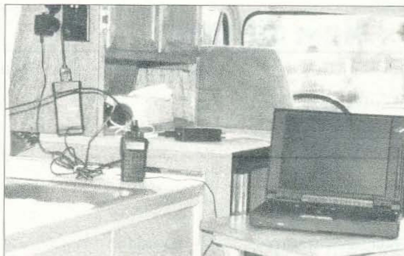
Photo A. Packet on wheels—Since the LDG Basic Packet Modem draws its power from the serial port of the computer, it is possible to run the entire packet station from batteries. Here, the battery providing power is the auxiliary battery of the RV. The modem is located just to the right of the ICOM W2A HT that is running without its battery attached. This makes the modem approximately the same dimensions as the radio. Two simple cable connections and your station is on the air. It was up and working at the time of the photo. The camera flash killed the screen display.
