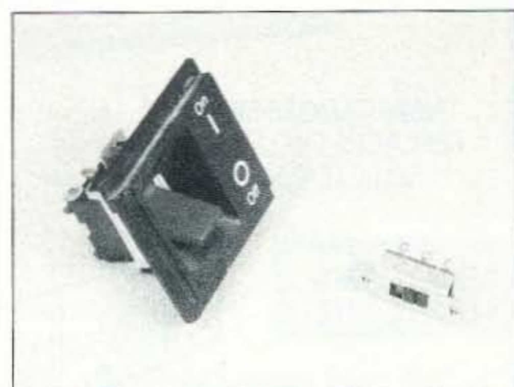
Photo C. The large plastic on/off switch was removed, and the hole sealed with an aluminum plate. The 120/240 VAC switch was removed and its wiring was bypassed, and the new on/off toggle switch was mounted in its place.
