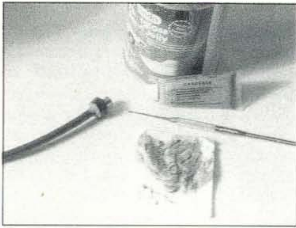
Photo C. After drilling the pilot hole for the center conductor, drill a hole in the cap equal in size to the diameter of the outer core of the HV wire insulator. Solder the center conductor of the HV wire to the interior of the cap, and then apply epoxy to the outer sheathing of the HV wire to ensure a good bond to the cap.
