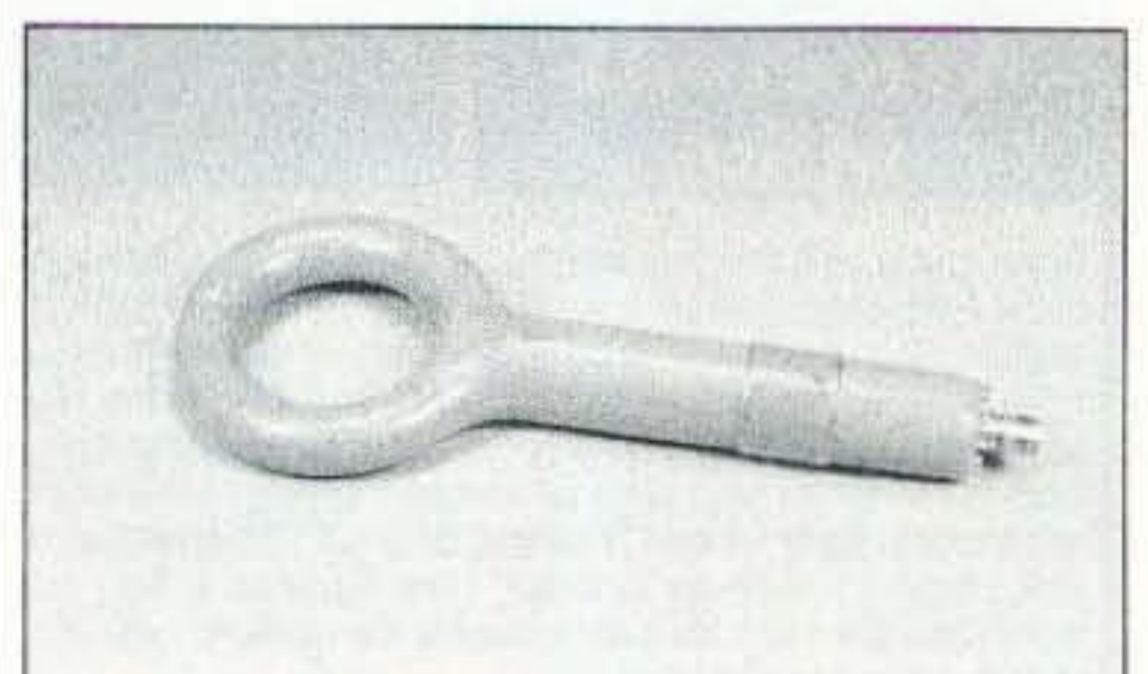
Photo B. EMI engineers use a probe like this to sniff out interference.
