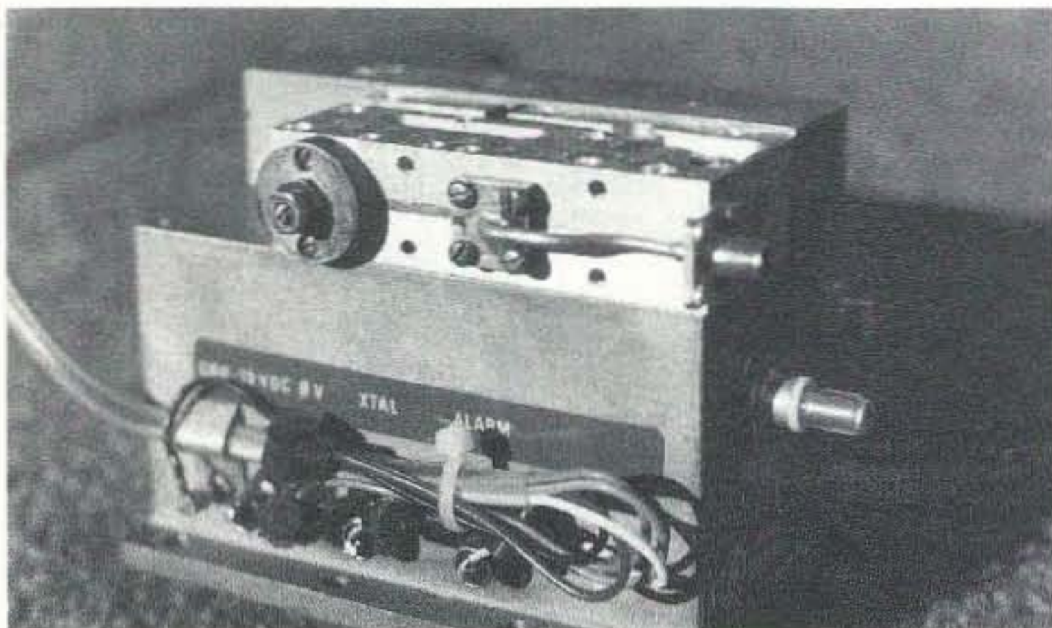
Photo A. Brick-type oscillator from Frequency West. Consists of a 100 MHz (approx.) crystal controlling a high-power oscillator at times 12 to phase-lock the unit. It then multiplies in a varactor to higher microwave frequency. (Multiplier not used when oscillator set up for 1152 MHz and 1296 MHz use.)
