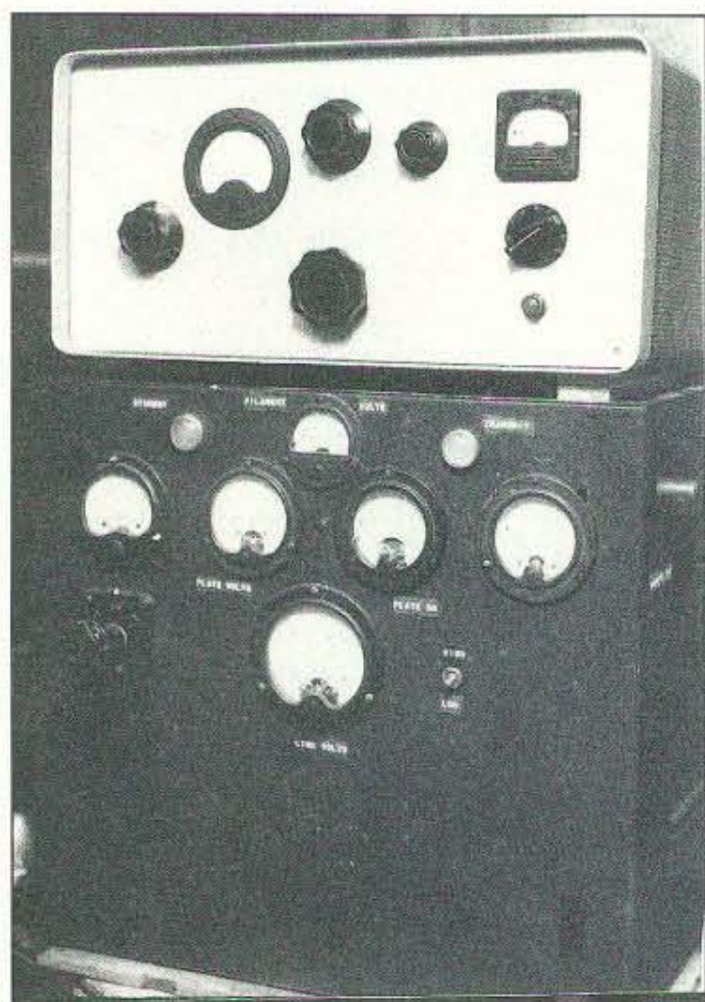
Photo F. The completed RF deck resting comfortably above a circa-1964 power supply. All voltages originate from the lower unit and must be cabled to the RF deck via quick disconnect assemblies.
