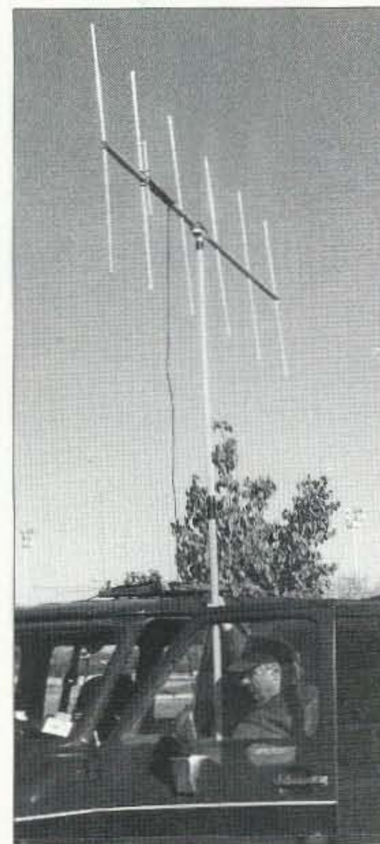
Photo E. Ron Racine VE2ESX needed this yagi antenna to get a bearing at the start point.
