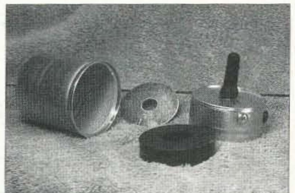
Photo A. Components of the Minnesota miser's magmount. (Photo by author.)
