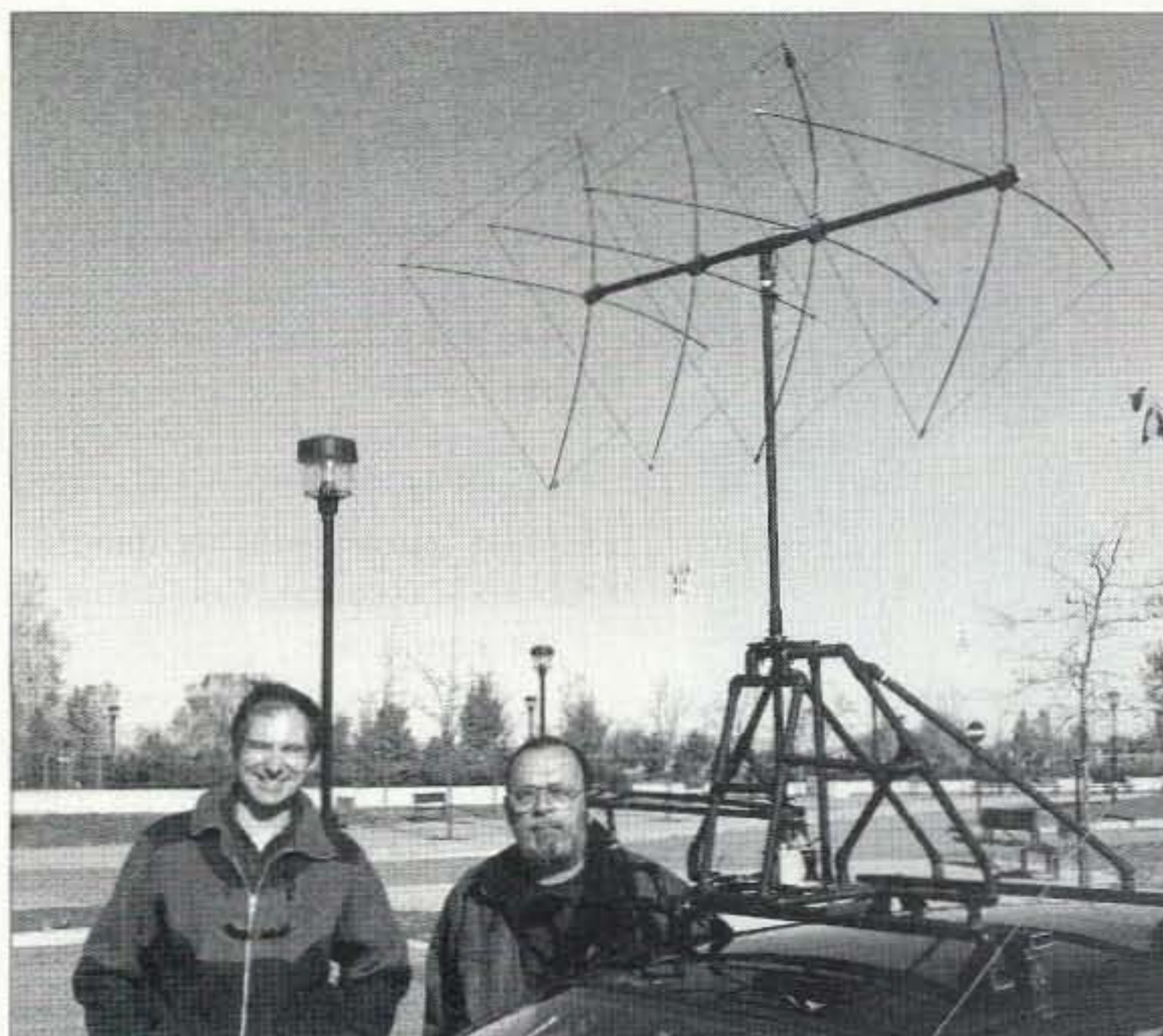
Photo D. This team has an elaborate rooftop mount for the two-meter mobile RDF quad, with a surplus radio-compass inside to indicate direction.
