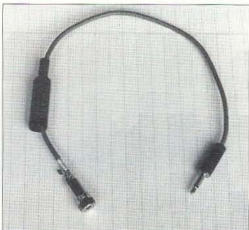
Photo D. Construction details of the ICOM CI-V adapter showing the 1N914 diode mounted inside the three-conductor 1/8-inch phone connector.
