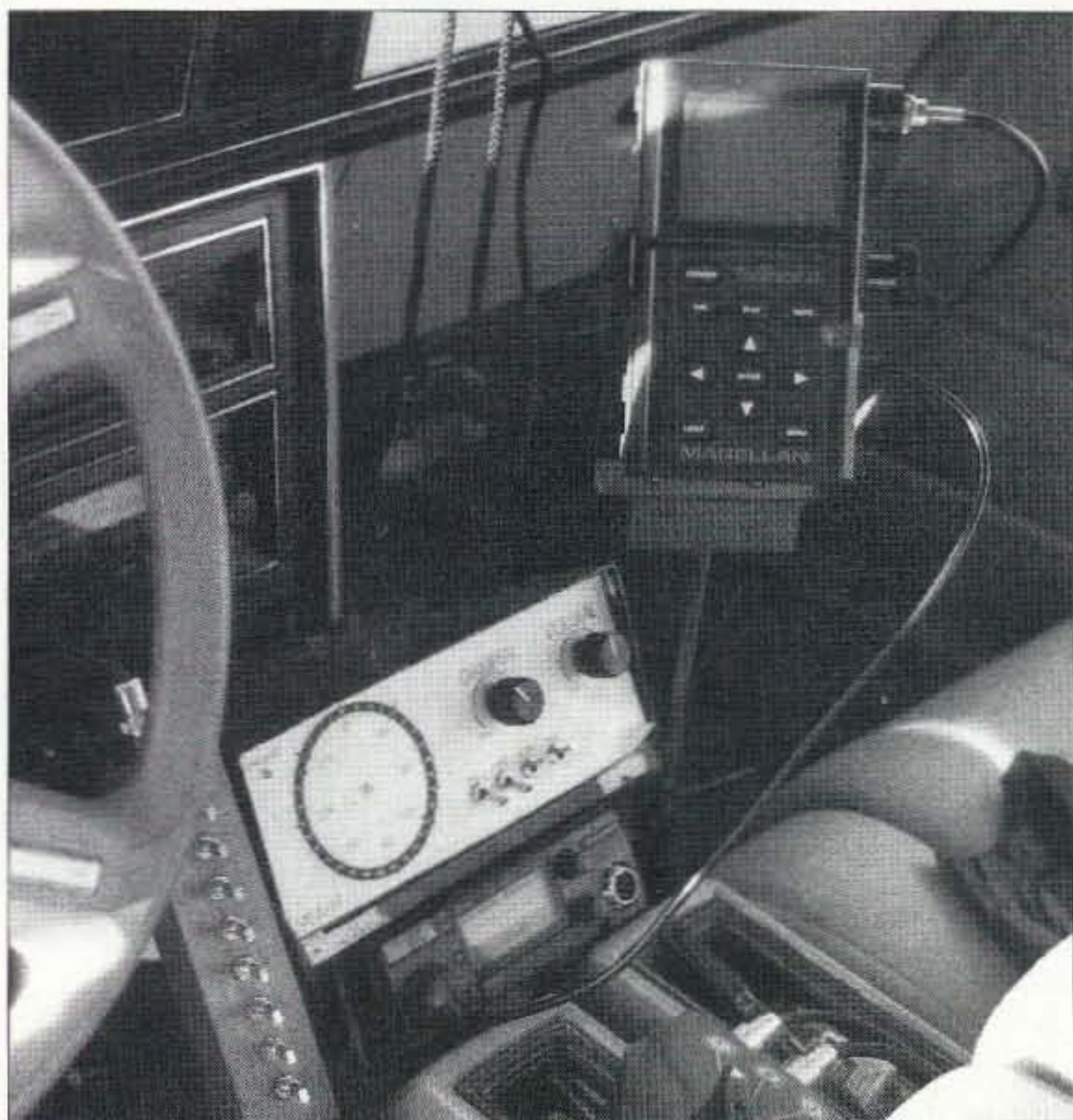
Photo B. Louis Tremblay VA2JX and daughter Viviane won the hunt using this mobile 32-LED Doppler setup. He also uses a GPS unit.
