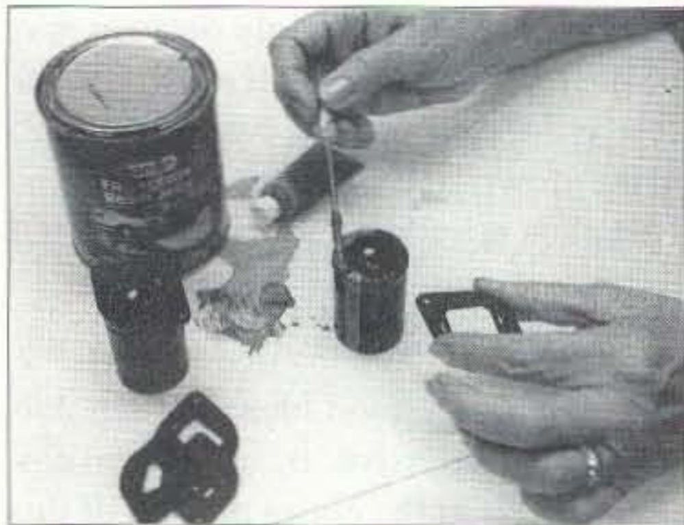
Photo D. Use some two-part epoxy to affix the phenolic wafer to the capacitor. Note that the banded end with the elongated zeros is the negative terminal. If care is exercised, the wafers can be recycled.
