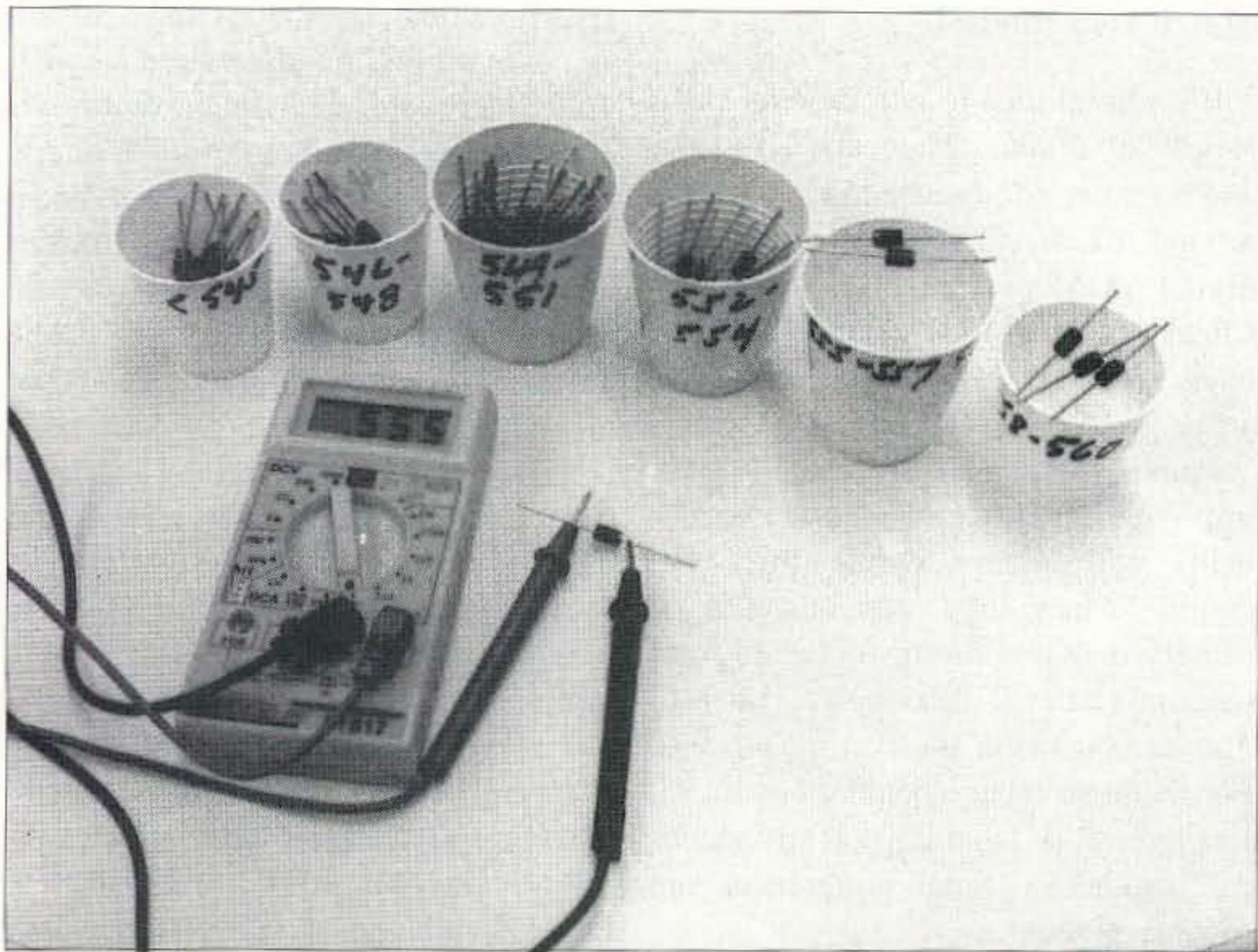
Photo B. It's a good practice to group power supply diodes by their value. In this case, the component with the .555 range readout will be placed in the second container from the right. Note how the majority of diodes cluster between .549-.551. Use this grouping for a long string of diodes in a full-wave bridge, since there are a sufficient number of closely related parts to complete the task.
