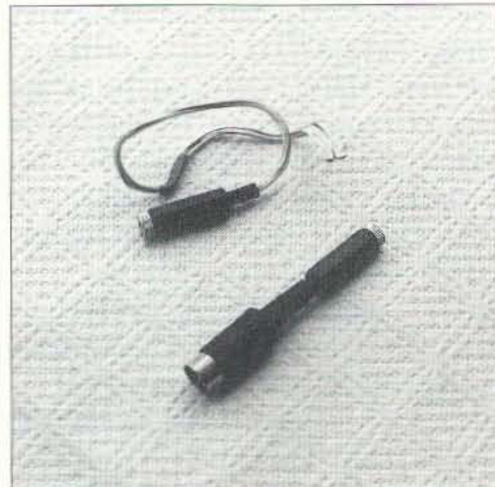
Photo E. Kenwood adapters for the basic universal interface circuit. The top adapter is used with a TS-50 by "pushing" the wire ends on to the pins of CN-6 (the TS-50's interface connector). The bottom one is essentially a plug adapter for Kenwood radios that use DIN-type interface connectors.
