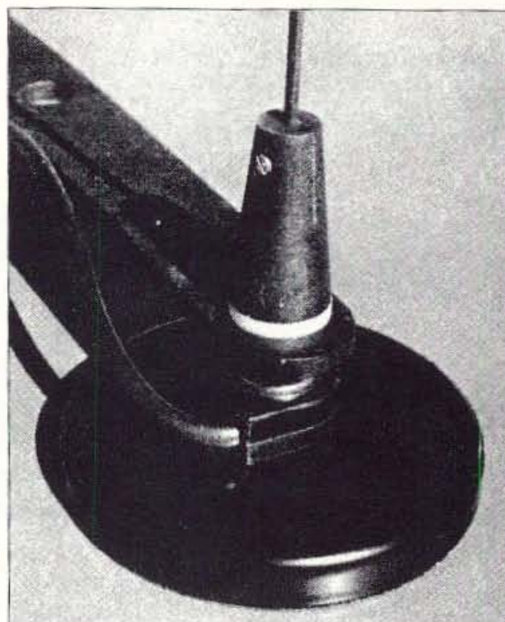
Photo D. The latest antenna set (fourth version) has a molded coax termination block to prevent shorts at the whip bases.
