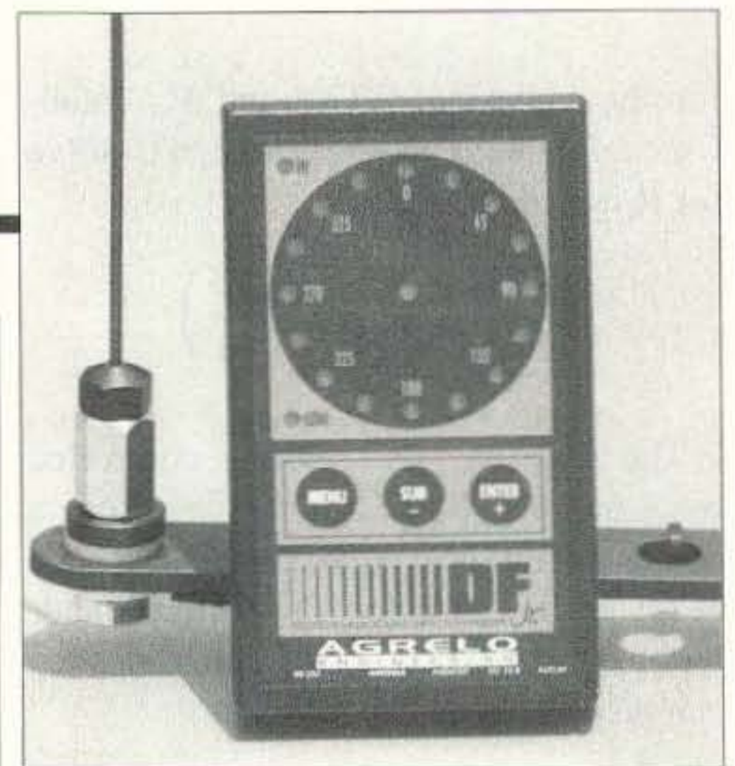
Photo A. The DFjr display box is about the size of a cigarette pack. Here it is next to one whip of the original version antenna set. All photos by author.
