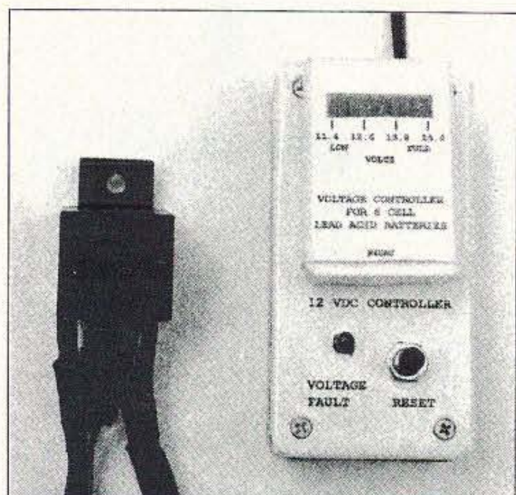
Photo A. Enhanced Automatic Voltage Controller with remaining 40 amp relay.
