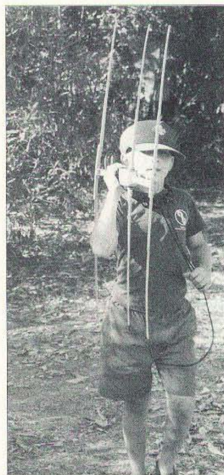
Photo C. To this Cub Scout, RDF gear seems a bit heavy after a few minutes of fox tracking. Next time, I'll add a mast so this Russian-made set can be held high more easily. (Photo by Joe Moell KØOV.)
