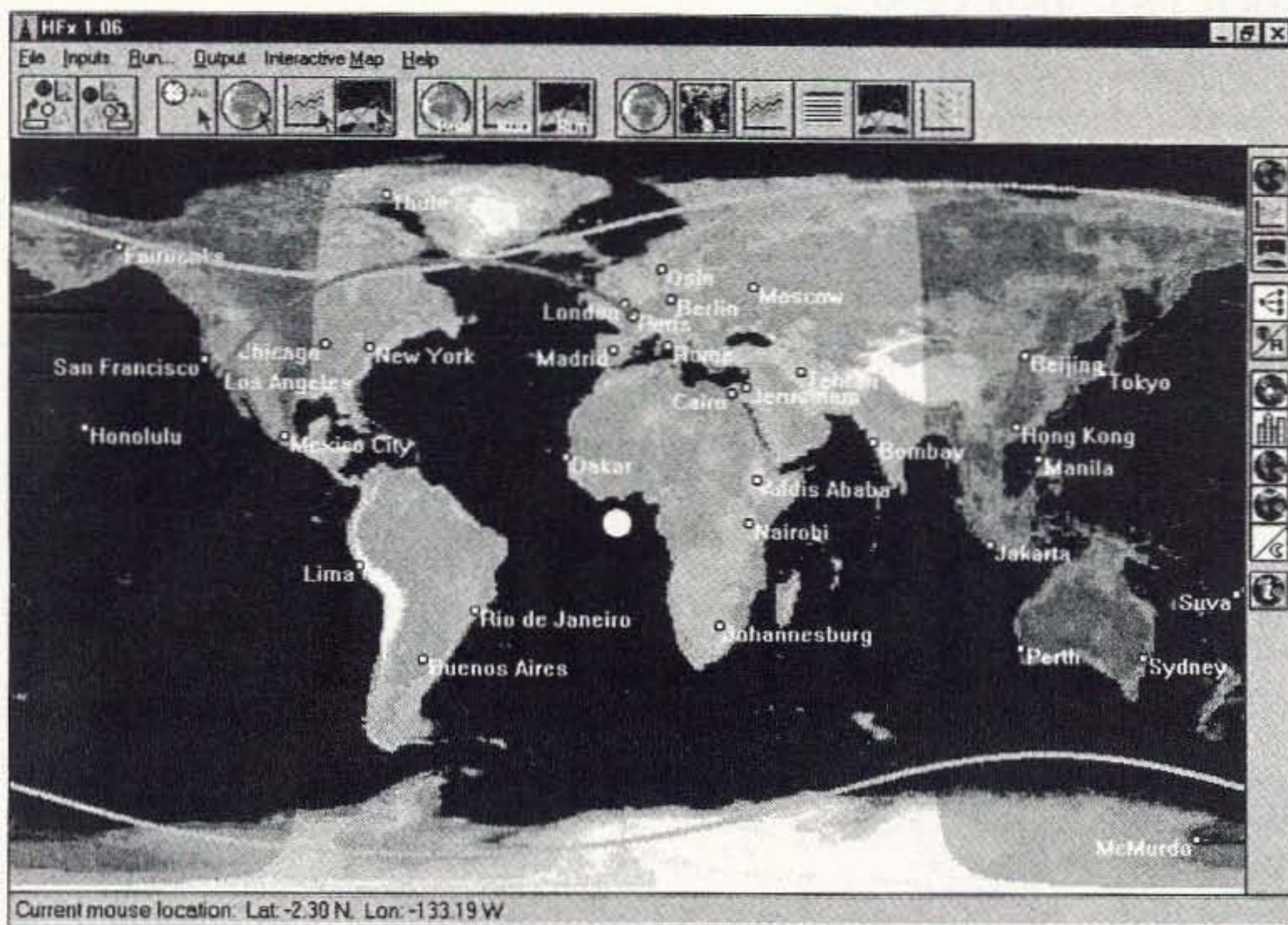
Fig. 6. Main screen, showing transmitting and receiving station placement, solar position, major world cities, great circle path between Tx and Rx, auroral boundaries based on geomagnetic activity and day/night terminator. These items may be turned on or off at user's discretion.
