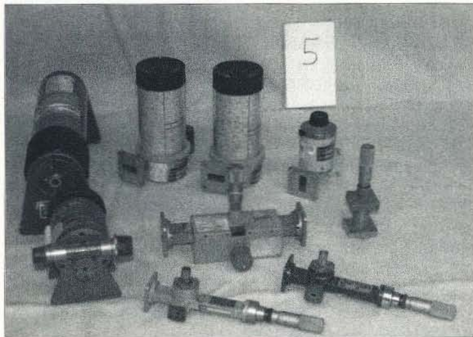
Photo A. Cavity wave meters (frequency meters) suitable for measurement at 10 GHz. The devices in the front row are slide-screw tuners, detector mounts and a sliding short for waveguide analysis.
