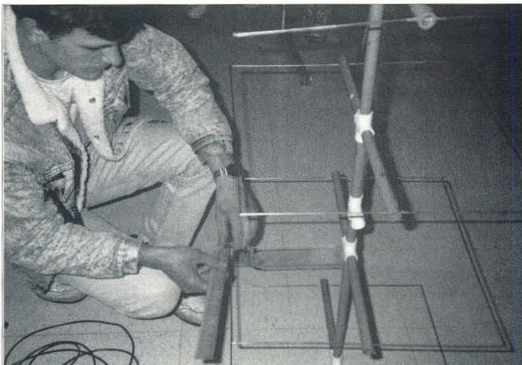
Photo B. Devin Corbett KB7NKT measuring the spacing for the feedline.
