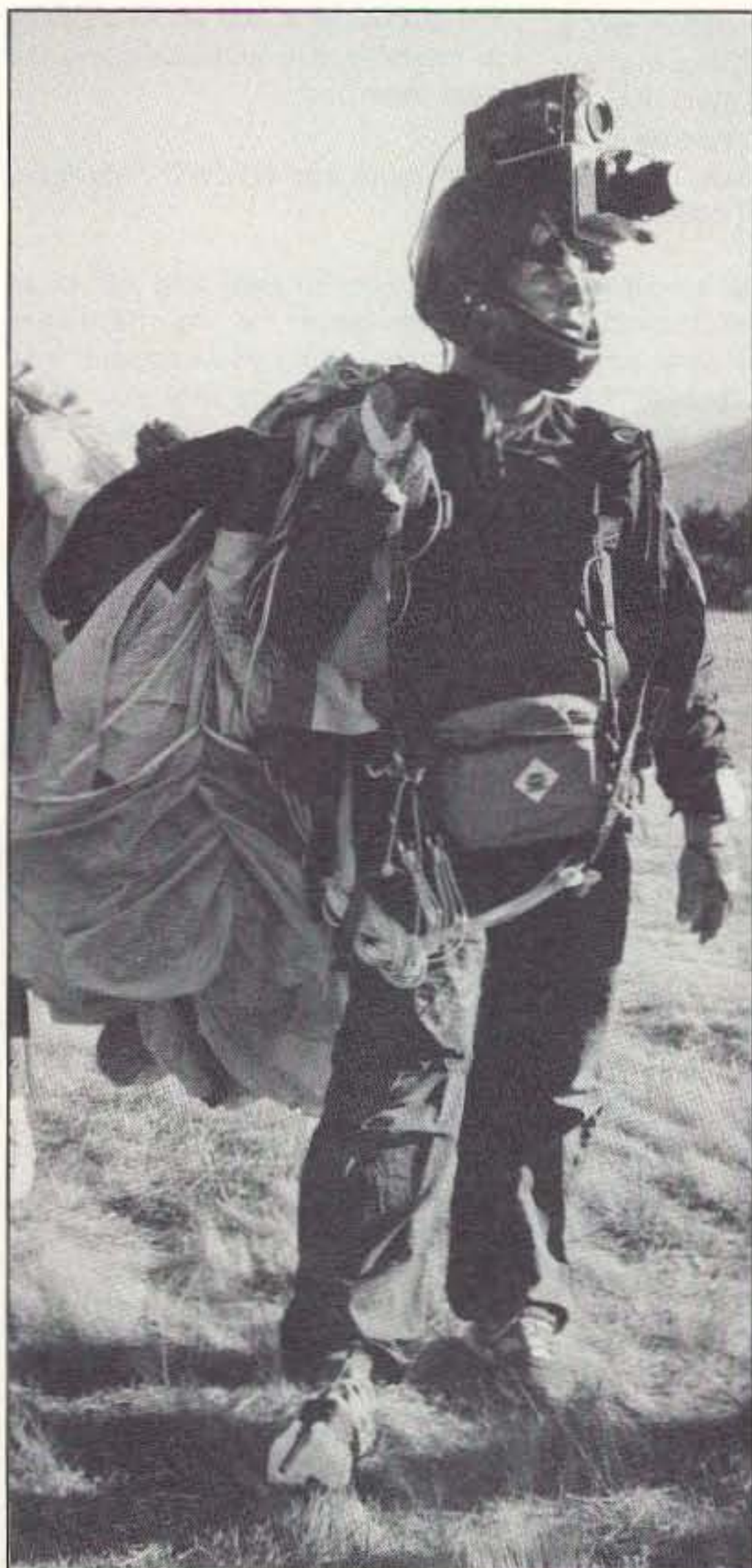
Photo A. Skydiver Jess Rodriguez demonstrates his unique helmet camera system complete with ATV transmitter. An 8mm camcorder and a 35mm film camera is mounted to his helmet via an aluminum bracket. The ATV transmitter is strapped to his waist inside of the knapsack and the ATV antenna can be seen attached to his shoe.
