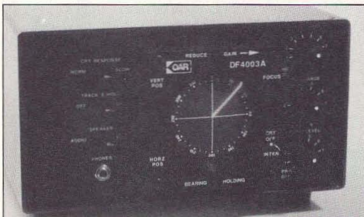
Photo A. Government agencies are the main customers for Watson-Watt RDF equipment from OAR Corporation. This Model DF4003A display unit works with external receivers and antenna sets covering 1 through 520 MHz.
