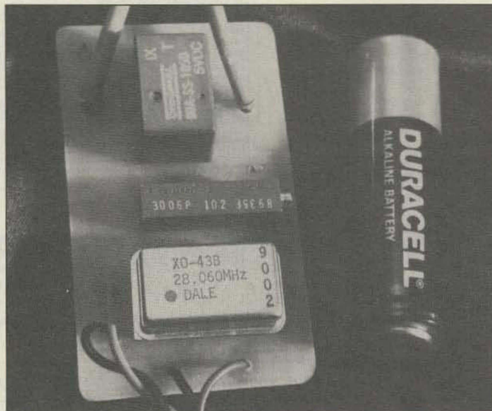
The FIRE-BALL, a battery-operated QRP rig, is powerful in the right hands. Note its size relative to the AA battery. (Photo by Elizabeth M. Devon.)
