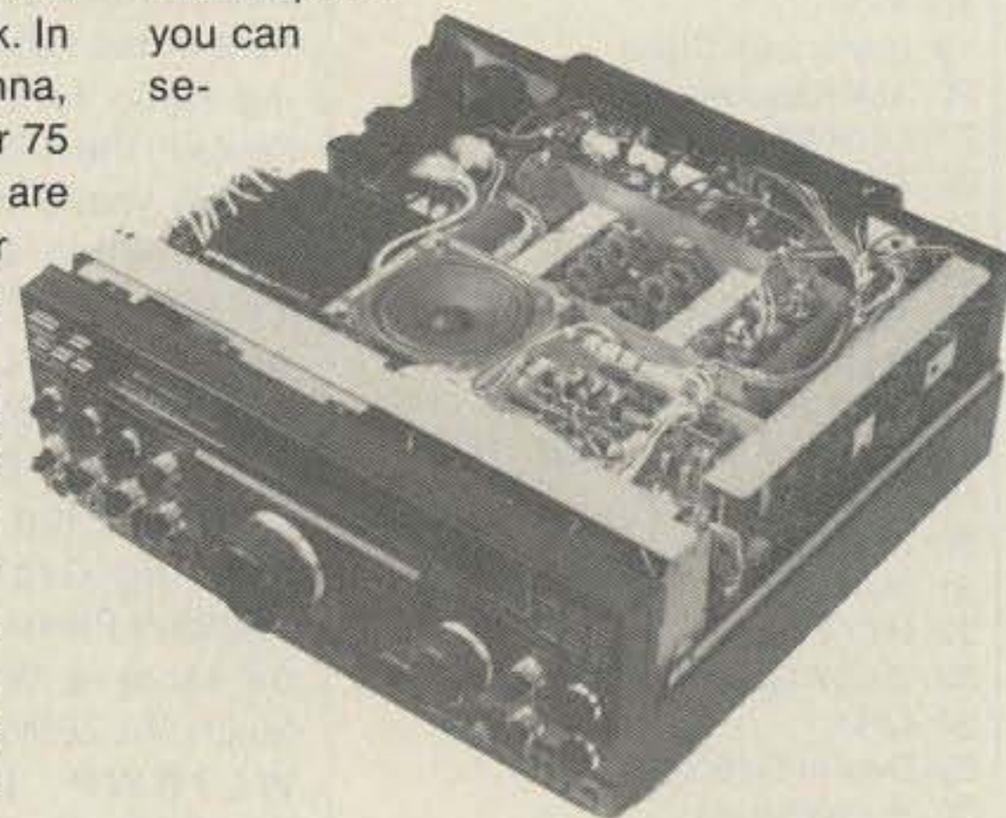
Photo B. Inside, the FT-1000 is stuffed with PCBs using surface-mount technology. Notice the large power transformer on the left.
