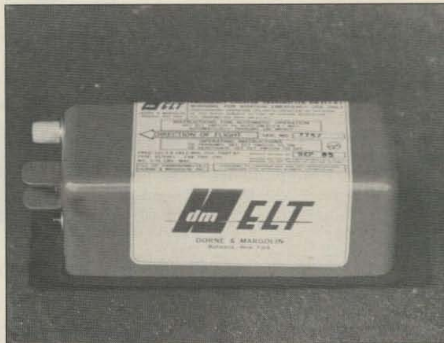
Photo A. This Emergency Locator Transmitter mounts in the tail of a small plane, and activates on impact. (Photo by WB6UZZ)
