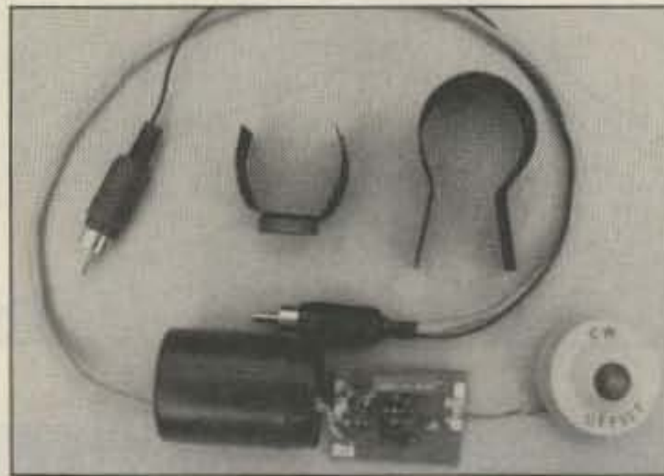
Photo A. The CW Offset Indicator, ready for installation. A 35mm film container makes an ideal housing.
