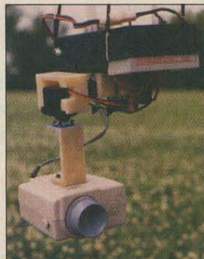
Photo C. Close-up view of the servo operated Az/EI camera mount.
