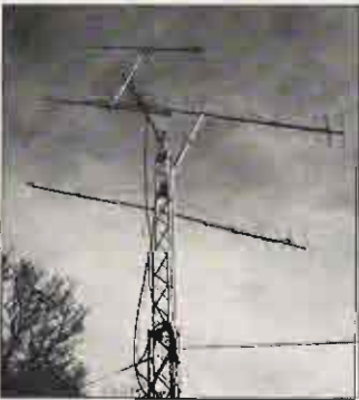
Photo A. Satellite antennas used at 4J1FS in late May for the DXpedition to Malyj Vysotskij (M-V) Island. (K7JA photo.)
