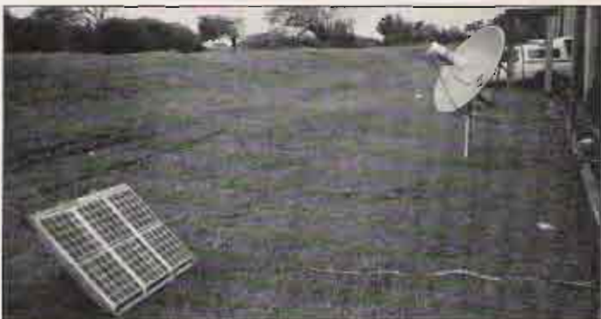
Photo C. Battery power with solar charging and Mode L operation with a four-foot dish at the N5EM Field Day site near Galveston, Texas. (N5LKJ photo.)
