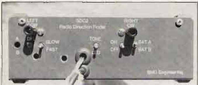
Photo B. Control panel of the SuperDF by BMG Engineering. WD6Y added these hoods to the LEDs on his unit to make them easier to see in bright sunlight, and drilled holes for access to internal controls.
