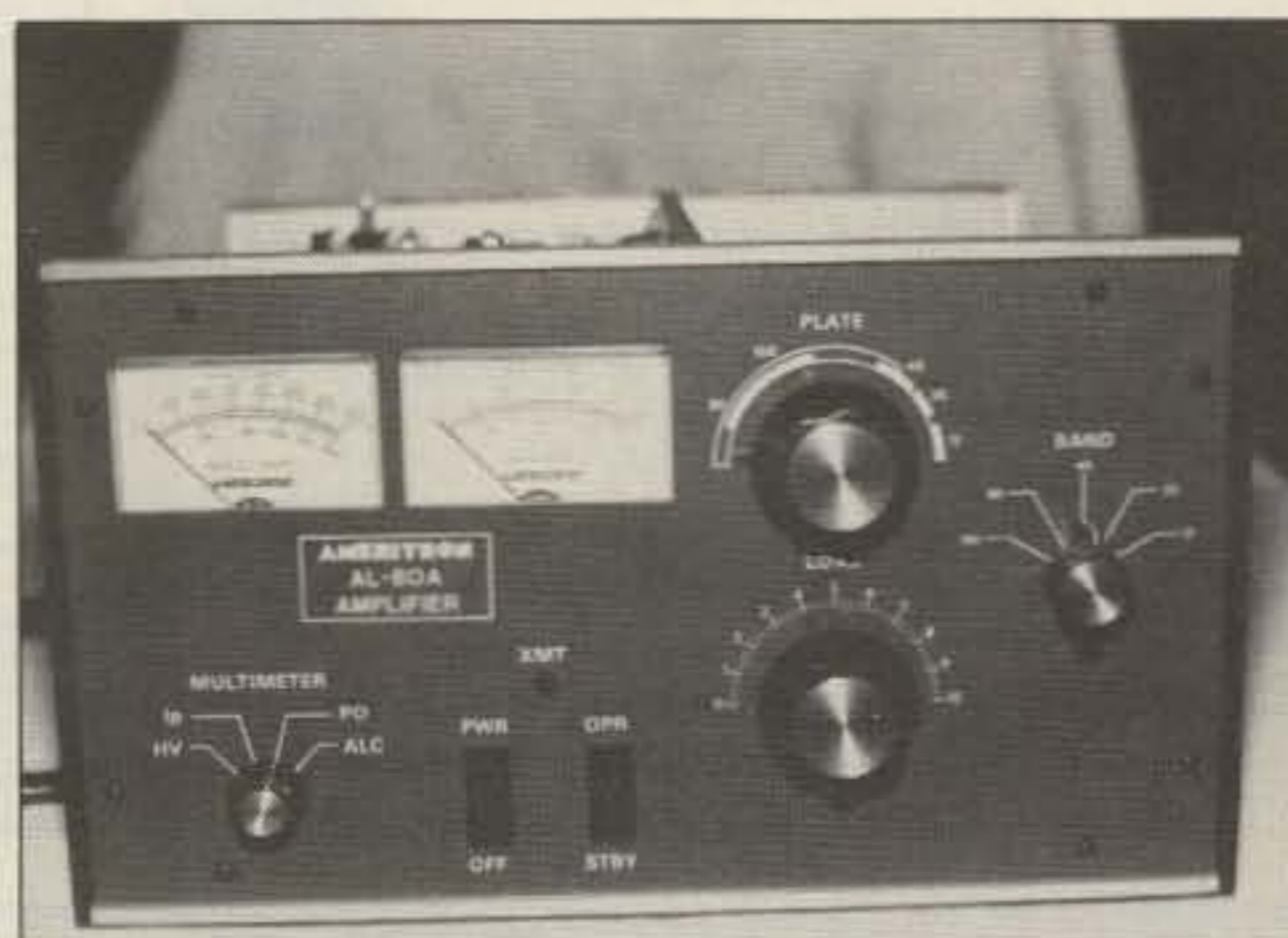
Photo A. The front panel of the AL-80A, showing controls, illuminated multimeter, and grid meter.
