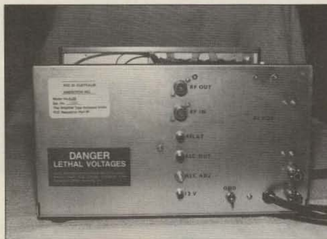
Photo B. Rear panel, showing the SO-239 connectors, phono plug connectors for RELAY, ALC OUT, and 12 VOLTS. Also visible are the ALC adjustment pot and dual fuses on the AC line.
