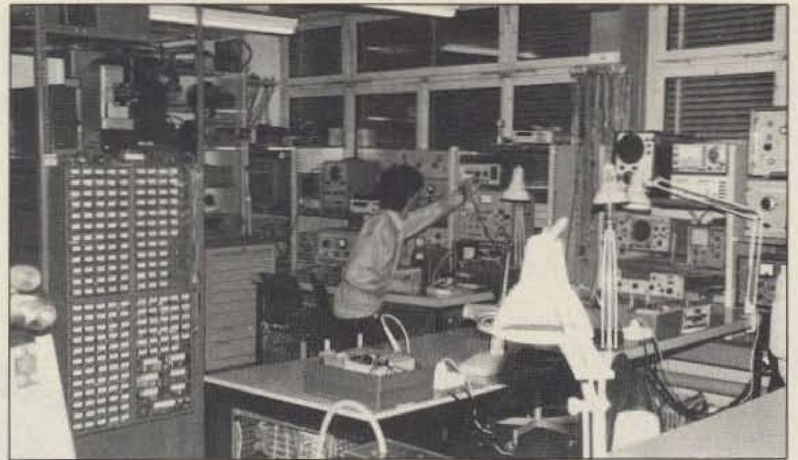
Photo C. At left are resistors and condensers; window shelves hold spectrum analyzer. Also shown are frequency generator (10 Hz to 12.6 GHz), frequency counters, and oscilloscopes.
