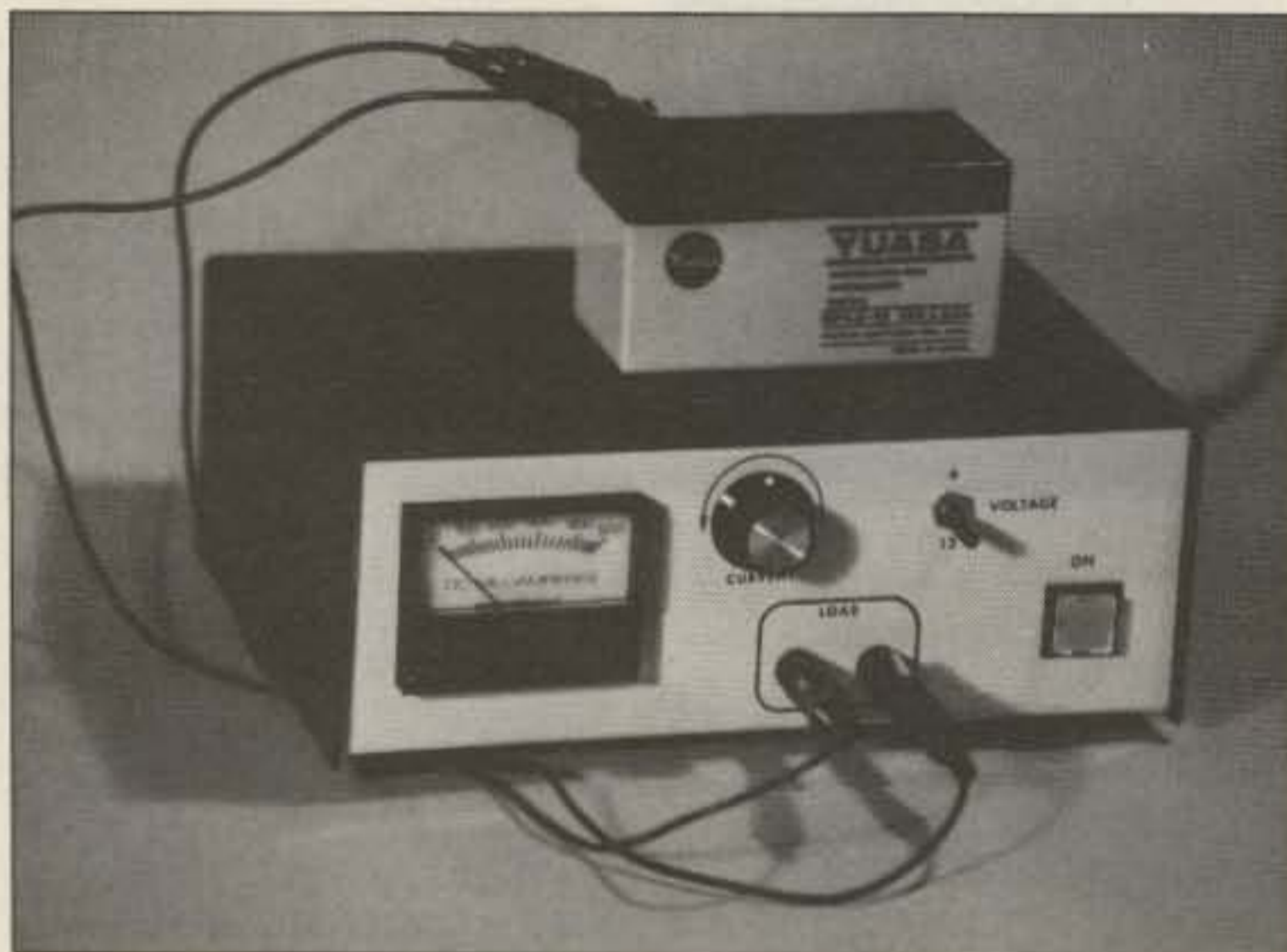
Photo A. The complete charger. Note the 0-500 mA panel for current adjust.
