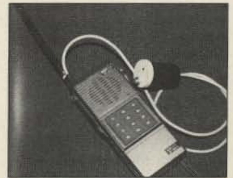
Photo A. A simple project, this external microphone adds mobile convenience to the ICQM IC-2AT.
