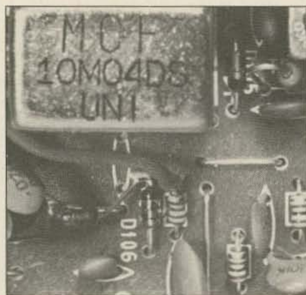
Photo A. Installation of the bypass section of the mod on the main board of the Uniden.
