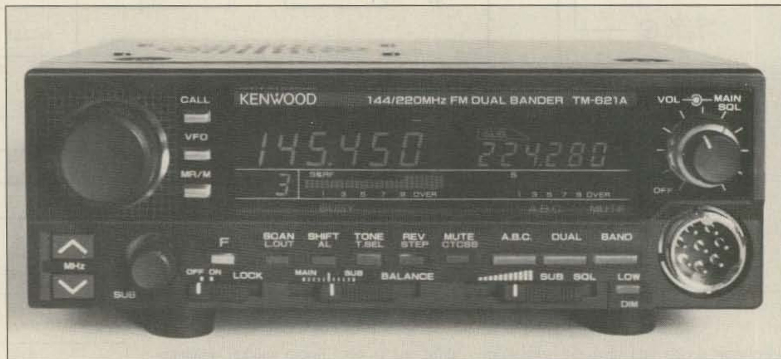
The Kenwood TM-621A—the world's first 2m/220 MHz dual-band mobile rig in a single box.
