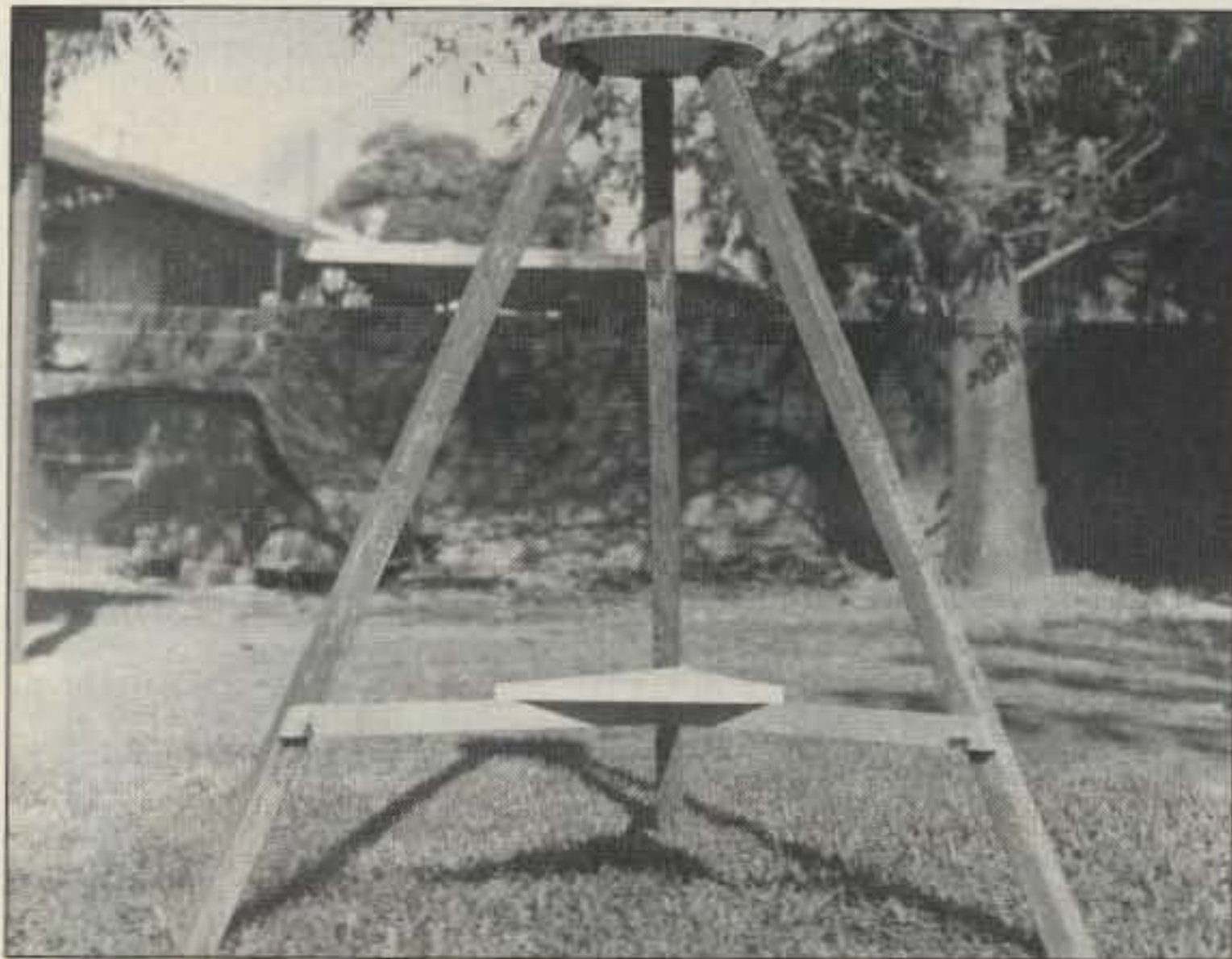
Photo A. Tripod construction with base stabilizer about one foot from the bottom end. Three hinges hold the three legs onto the wood base.
