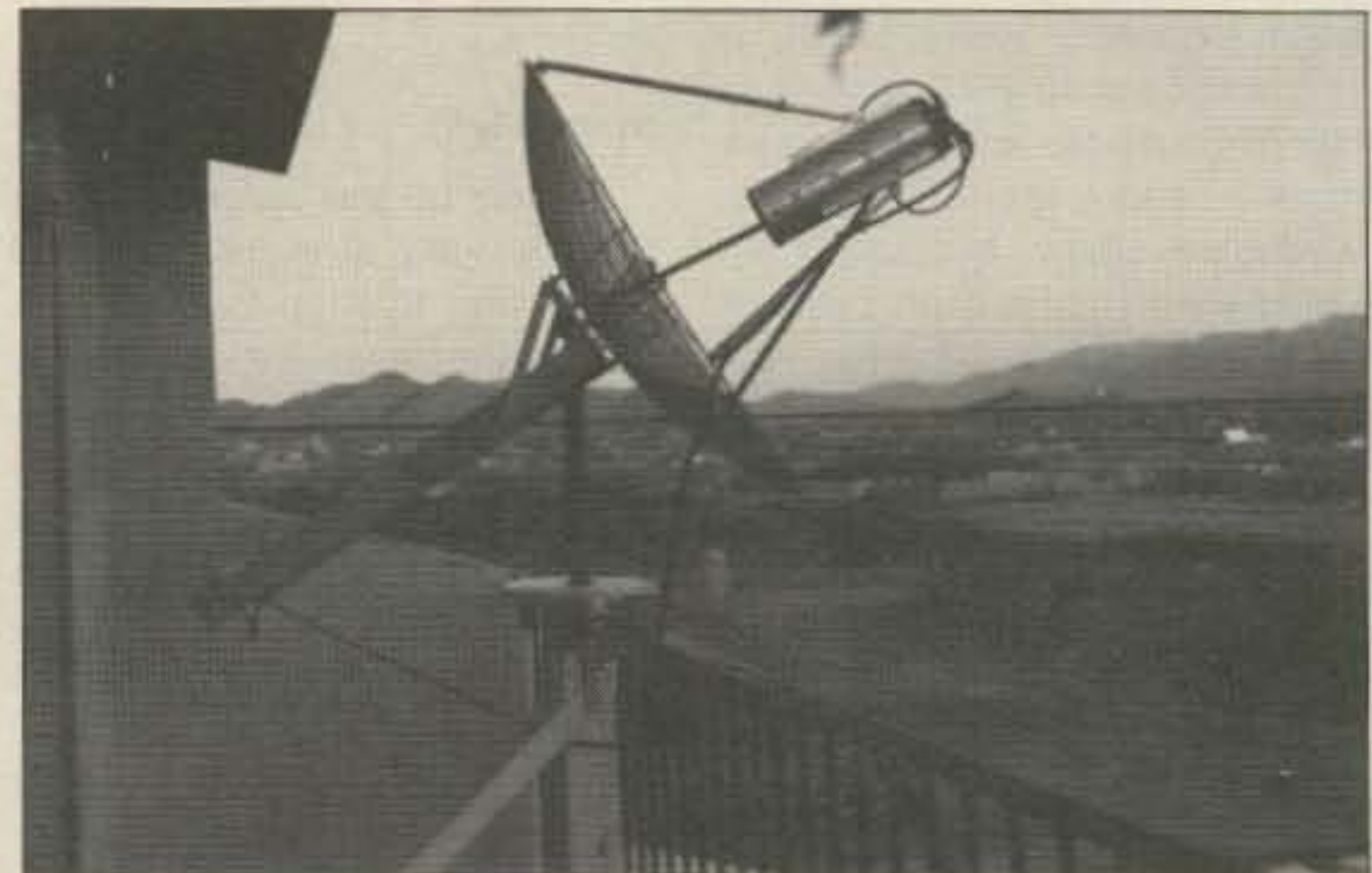
Photo D. Four-foot dish with coffee-can feed for Mode L uplink at W6ABN.
