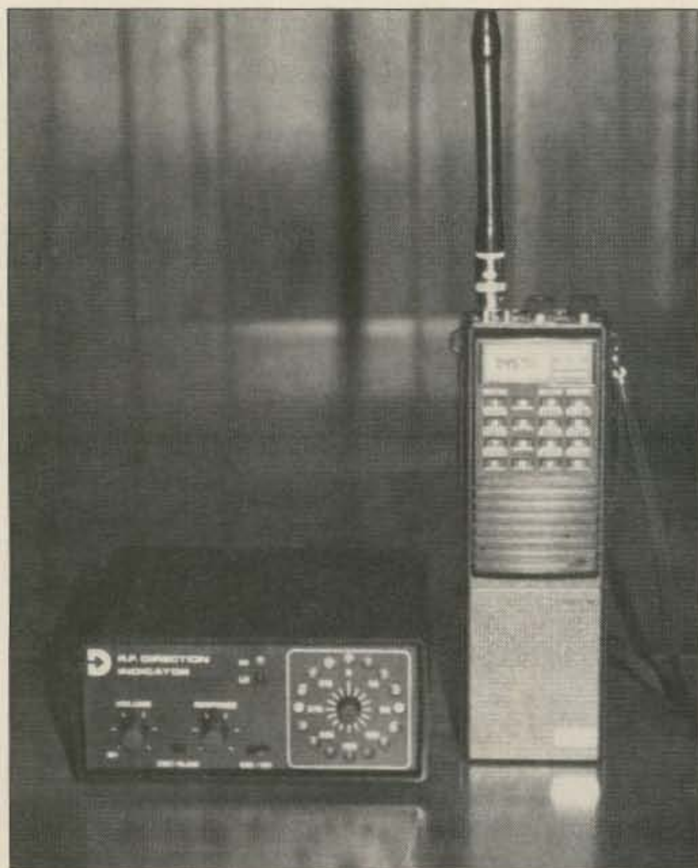
Photo A. The DF display unit. Note the circle of 16 LEDs on the front panel at left. Each represents 22.5 degrees of azimuth.
