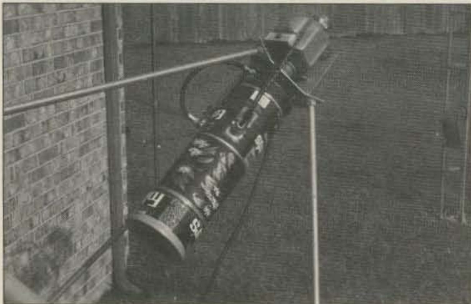
Photo C. Close-up of the coffee-can feedhorn on the six-foot dish.
