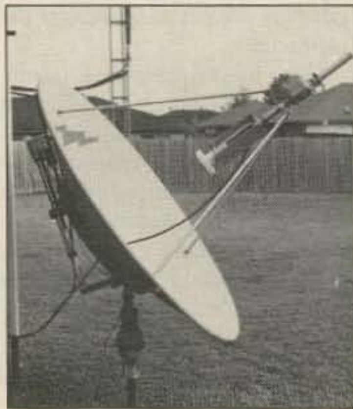
Photo A. Six-foot TVRO system with separate azimuth and elevation control.
