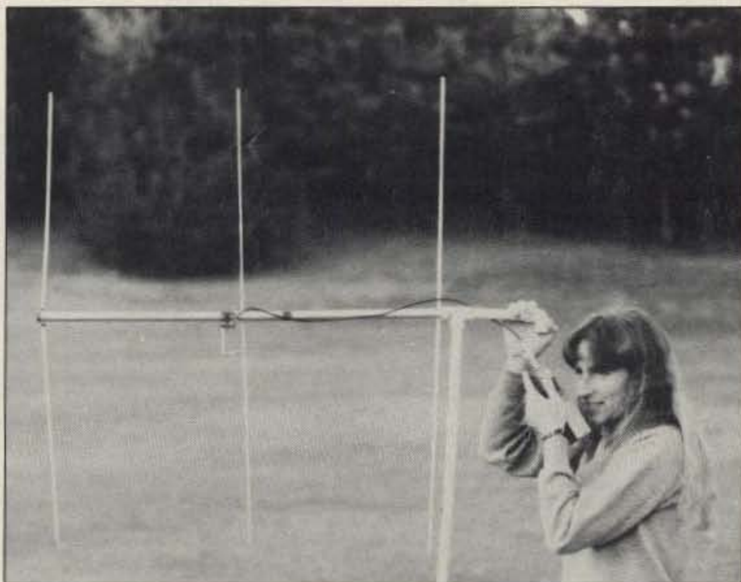
Photo B. The assembled portable Yagi in action.
