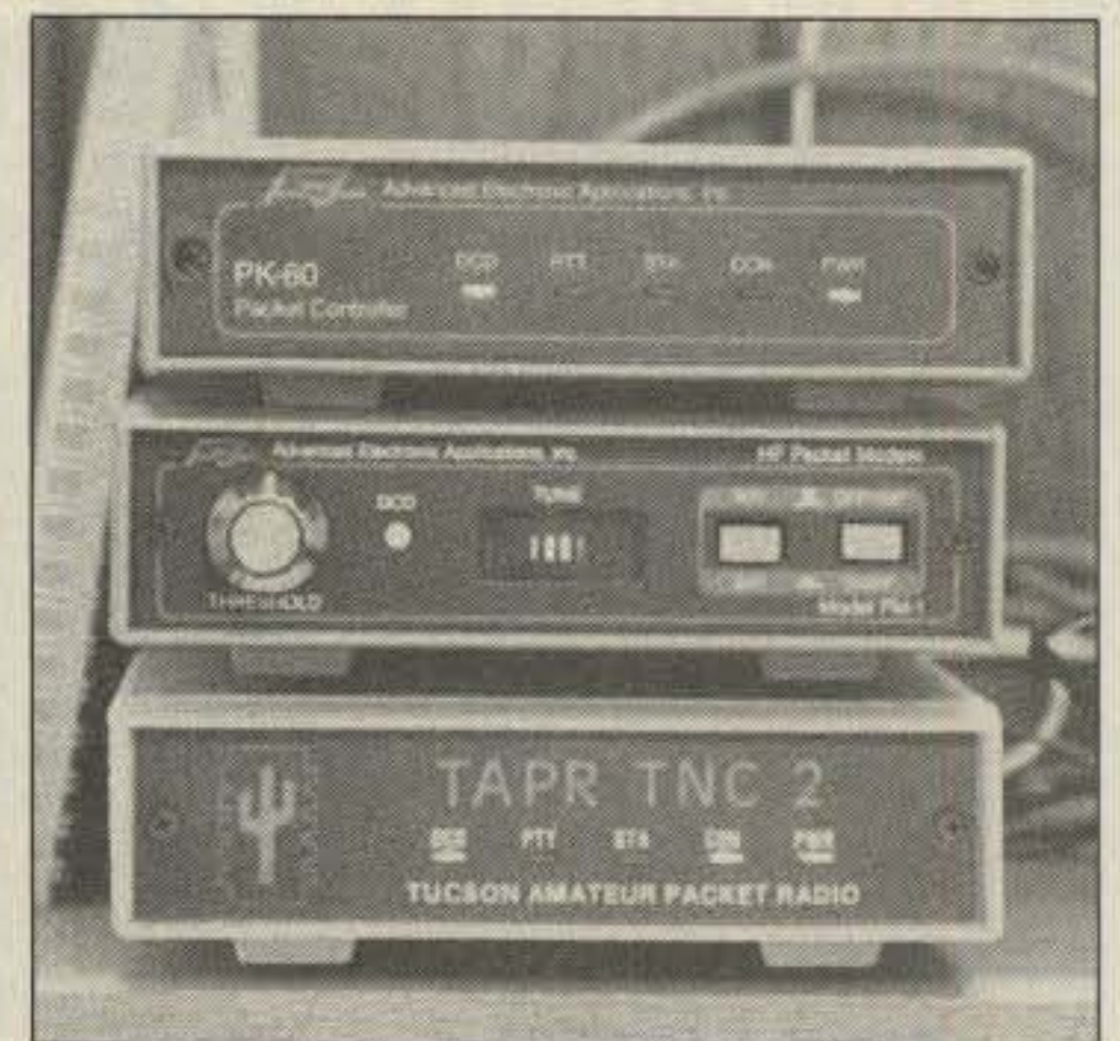
Photo B. Closeup of the station pictured in Photo A. The center box is the AEA PM-1 HF modem. Many HF stations are discovering that a modem optimized for HF operations makes a big difference in the number of packets heard without retries. Modified RTTY TUs have also been used with success. The modem included with most TNCs is either a generic PLL-type design or a modem chip designed for telephone use. In some cases, performance of these modems on a noisy HF link is marginal.
