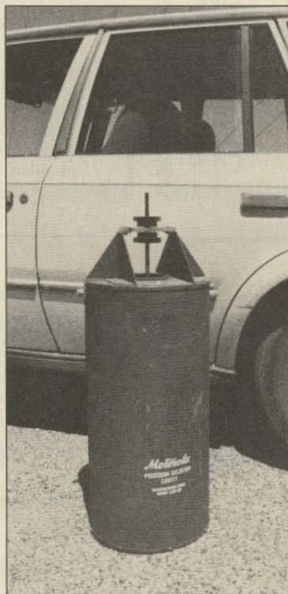
Photo B. A two-meter pass cavity is much like an antenna: If it is small enough to be convenient, it is too small. This one is 24" tall and 9" in diameter.
