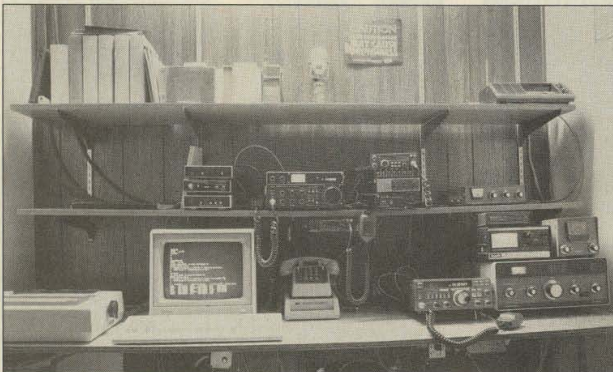
Photo A. Typical W0RLI/WA7MBL BBS and gateway station. The station includes an IBM-PC clone, two TNCs, a VHF radio, and an HF radio. This is WB6KAJ-1, run by Lee Dusbabek.
