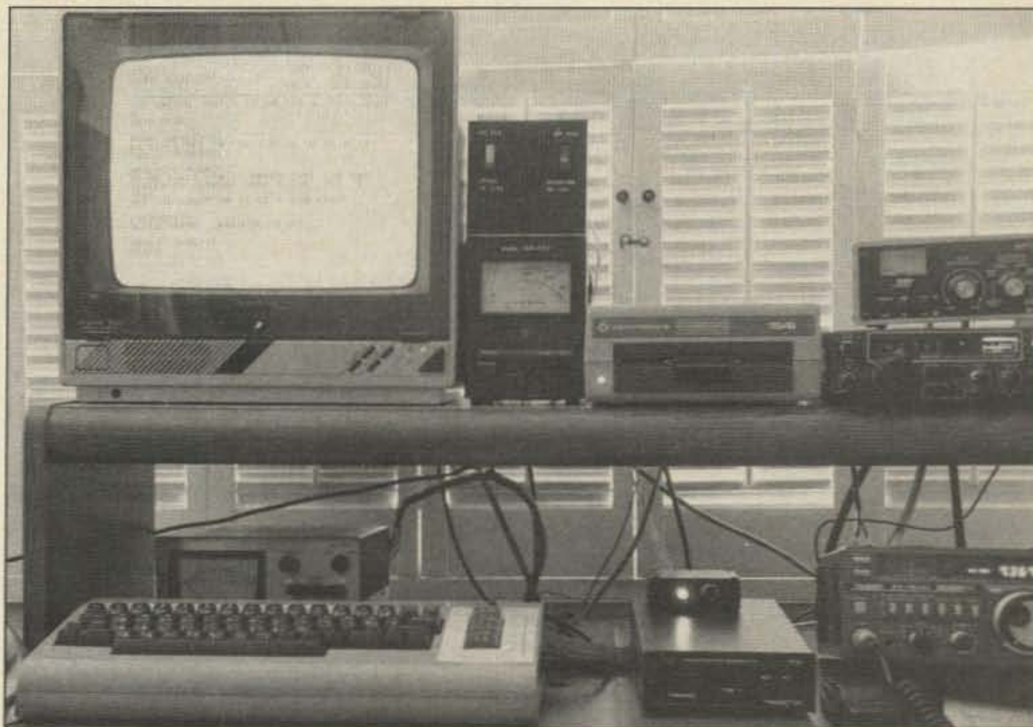
Photo A. One of the more common types of packet stations among new packeteers is the Commodore-64 based system which uses either a stand-alone TNC or a unit specially designed for the C-64—like the one pictured here, AEA’s PK-64. This station belongs to Colin Hall, G4JPZ/W6. It features (top to bottom, left to right): CRT, antenna rotor, C-64; antenna switches, antenna rotor; C-64 disk drive, power switch for PK-64 (home-brew), PK-64; HF tuner, VHF radio, HF radio.
