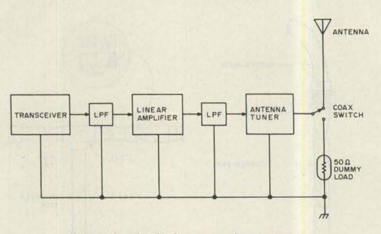
Fig. 8(a). Block diagram of my station.
