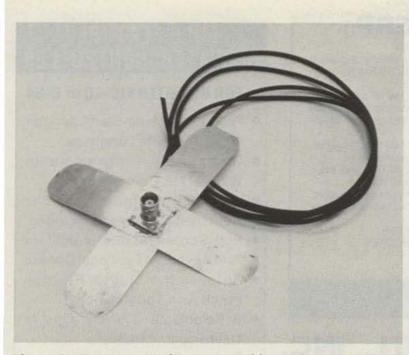
Photo C. Connector and strip assembly ready to be placed inside of the hat. Be sure the coax can reach at least to waist level.
