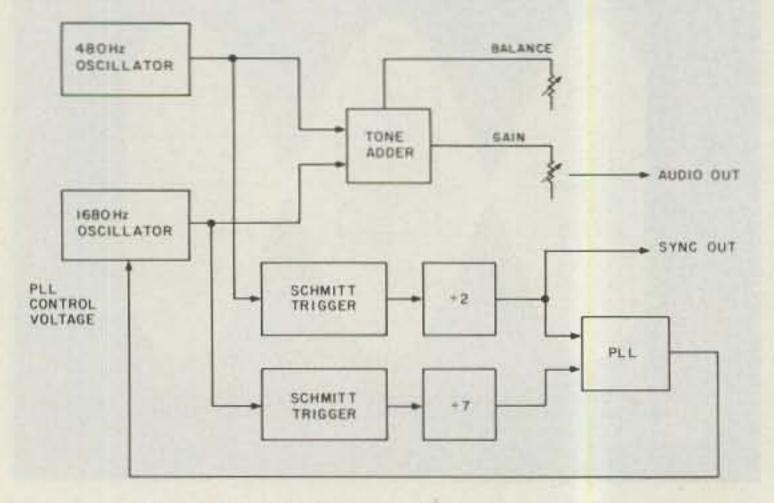
Fig. 3. Block diagram of Two-Tone Plus. 38 73 for Radio Amateurs • April, 1985 most transceiver designs.
