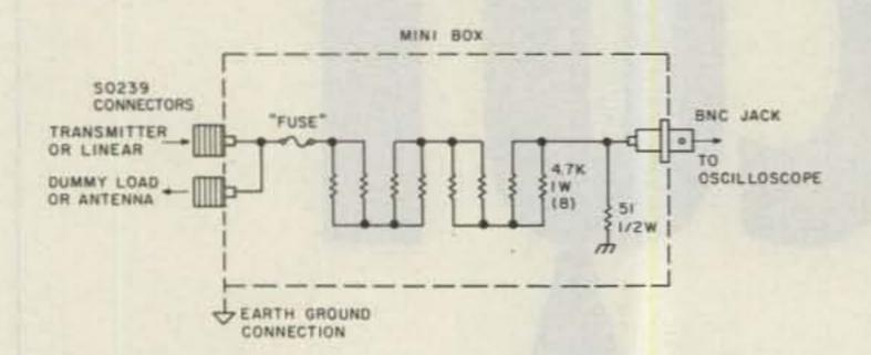
Fig. 8. L-pad power sampler. All resistors comp. or film (noninductive). Fuse is thin copper strand from zip cord, 1/2" to 3/4" long. Connect SO-239 connectors with RG-8 center conductor wire. Keep BNC connector 3" away from SO-239s; space resistor sets 3/8" apart. Test run sampler at full power before connecting to scope. Maximum power 2 kW PEP; 1 kW CW. Maximum vswr 2:1.
