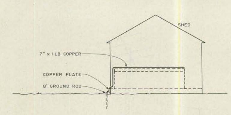
Fig. 9(a). Method of bringing the copper flashing outside.
