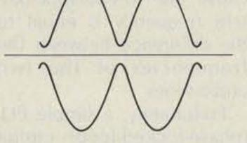
Fig. 2(f). Pattern due to unbalanced tones (not amplifier problem).
