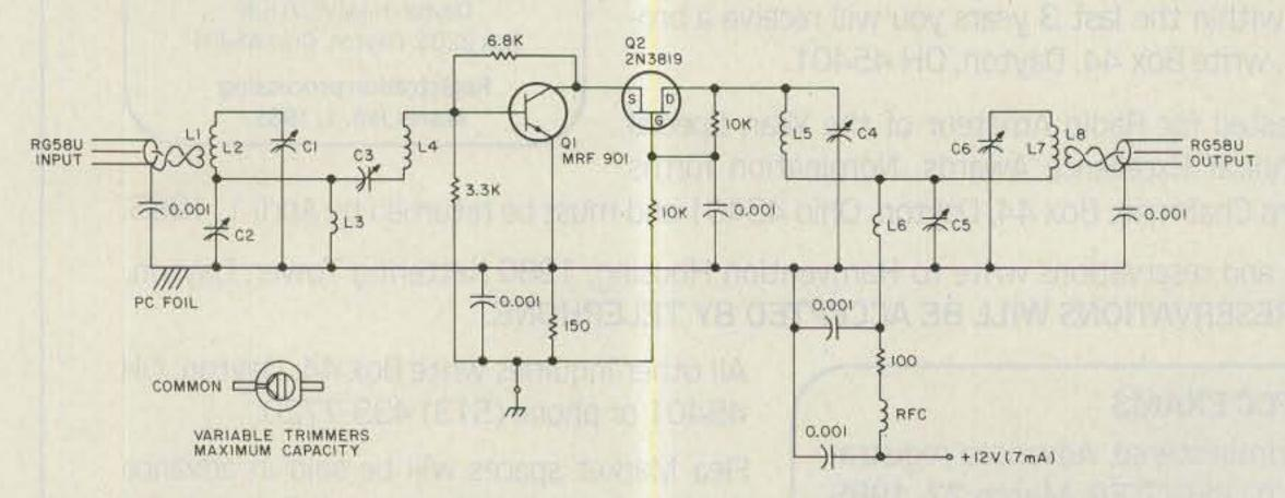
Fig. 1. Schematic diagram of the preamplifier. Numbered components are identified below. Fixed-value resistors are carbon composition, 1/4 W. Fixed-value capacitors are disc ceramic, 50 WV. Numbers in parentheses identify Radio Shack numbers.
