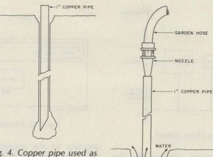
Fig. 4. Copper pipe used as a ground rod.
