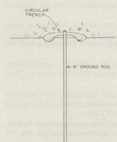
Fig. 3. A method for improving ground-rod effectiveness in very dry or sandy soil. is to reduce the impedance as much as possible. The resistive component of this impedance is mostly the resistance between the ground rod and the earth. Therefore, the biggest improvement comes from increasing the surface area of the ground rod that is in contact with the earth. This is the main reason why we want the ground rod to be driven in all the way and its length to be 8 feet.
