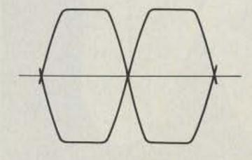
Fig. 2(c). Overdriven amplifier pattern.
