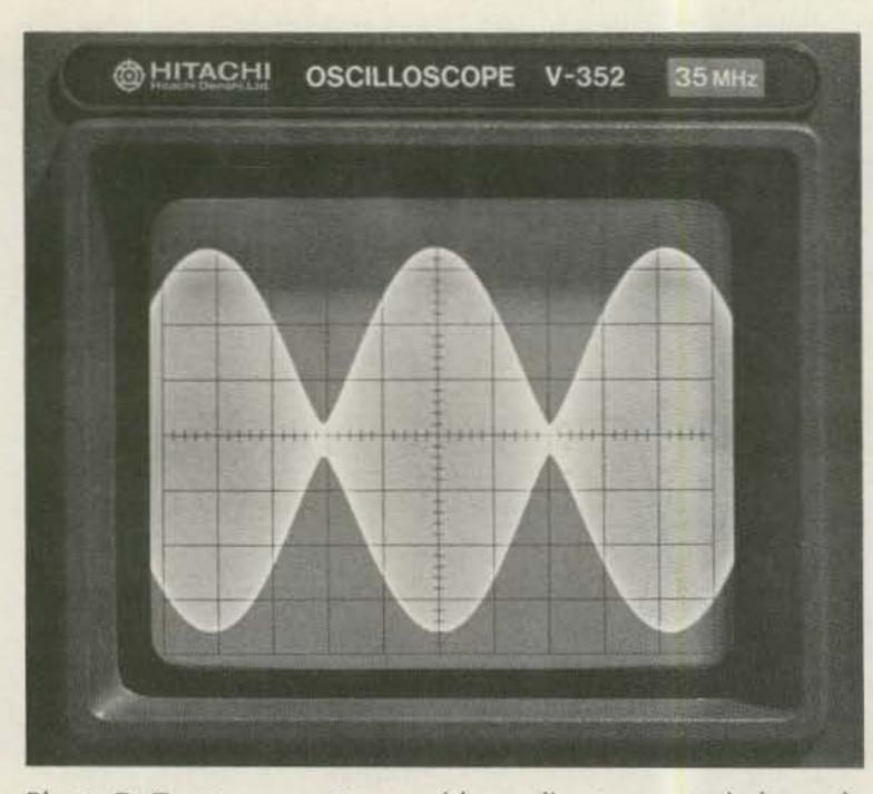
Photo D. Two-tone pattern with audio tones unbalanced. Not an amplifier problem! Always adjust the Balance control for a complete null.
