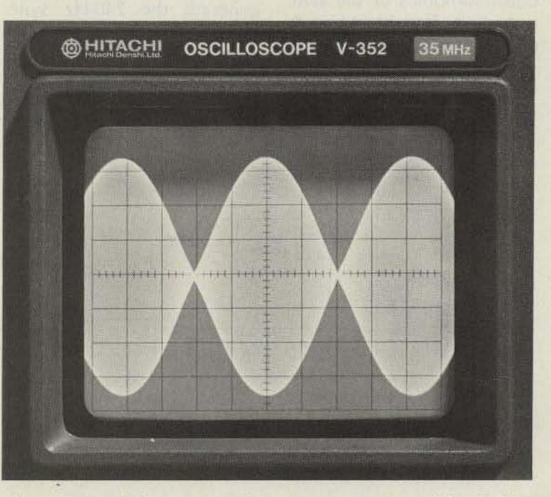
Photo C. Typical two-tone rf test pattern. Note stable display. 73 for Radio Amateurs • April, 1985 37
