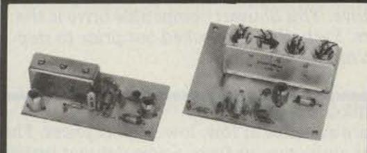
Our lab has developed a new line of low-noise receiver preamps with helical resonator filters built in. The combination of a low noise amplifier and the sharp selectivity of a 3 or 4 section helical resonator provides increased sensitivity while reducing intermod and cross-band interference in critical applications. See selectivity curves at right. Gain = approx.12 dB.
