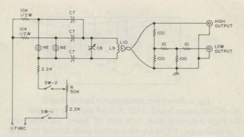
Fig. 3. Schematic of the power-line noise source. Numbered components are identified below. Fixed-value resistors are carbon composition, 1/4 W unless otherwise noted. Numbers in parentheses identify Radio Shack numbers.
