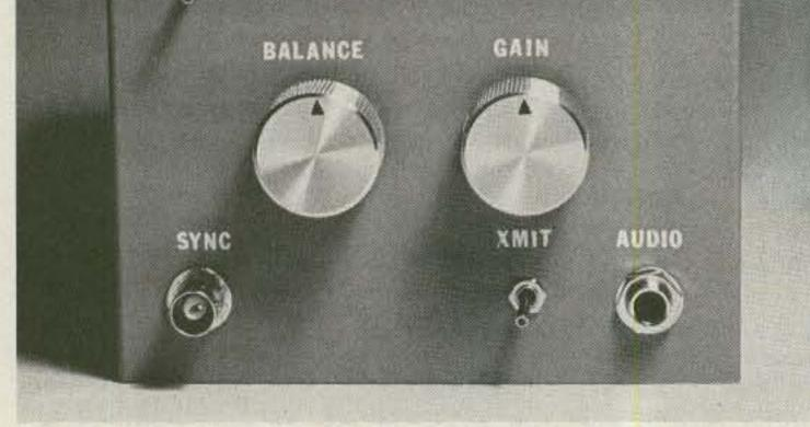
Photo A. Two-Tone Plus is an SSB-transceiver and linear-amplifier tuning aid which includes a sync output for stable rfwaveform viewing.
