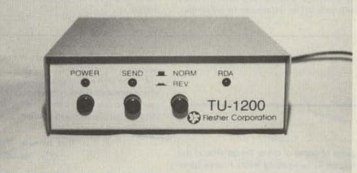
Photo A. The TU-1200 VHF/UHF RTTY Interface from Flesher.
