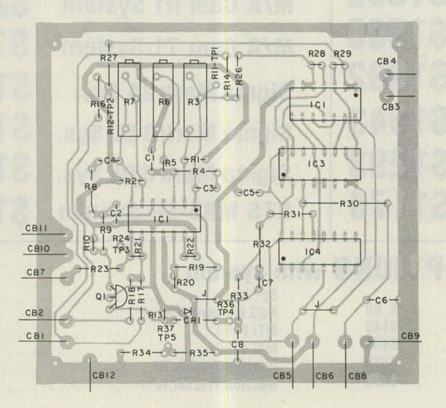
Fig. 7. PCB parts placement.
