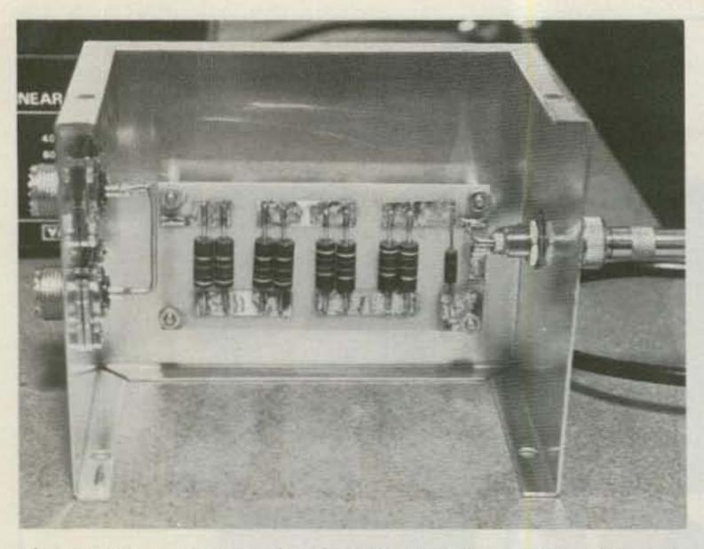
Photo G. Construction detail of the L-pad sampler. Although simple, build the L-pad carefully since it handles high power.
