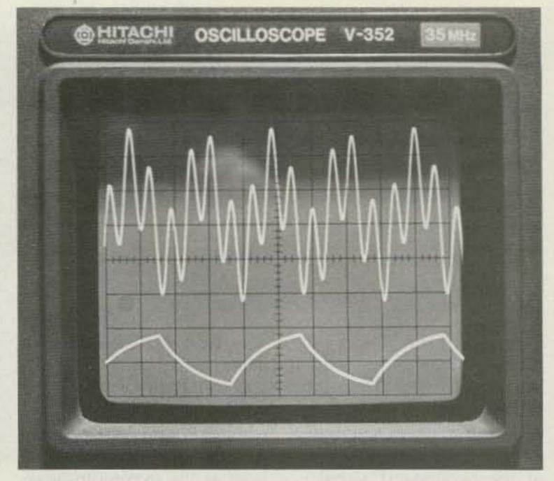
Photo E. Upper trace shows the composite audio output of the Two-Tone Plus generator. Tones are synchronized but are not harmonically related. Lower trace shows sync waveform. Both tones are harmonics of the sync frequency.
