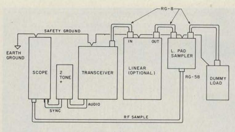
Fig.1. Two-tone test setup, top view.
