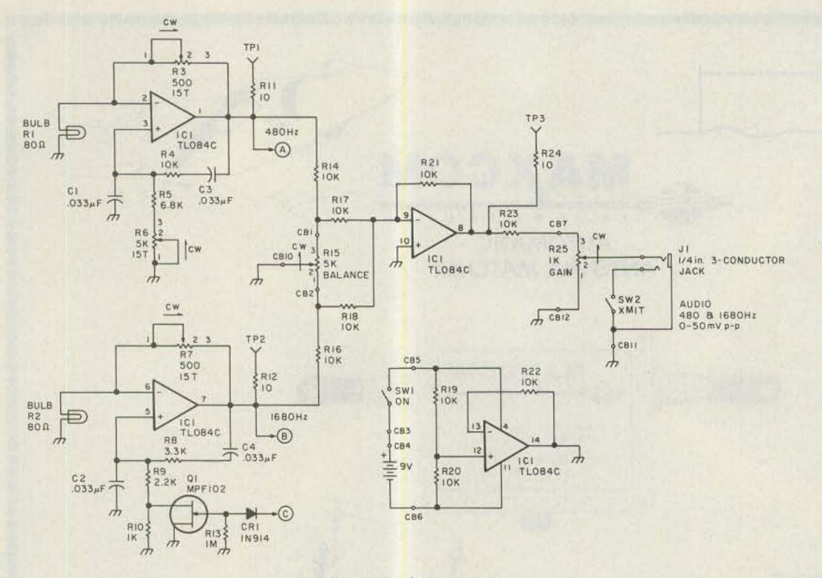
Fig. 4. Analog section.
