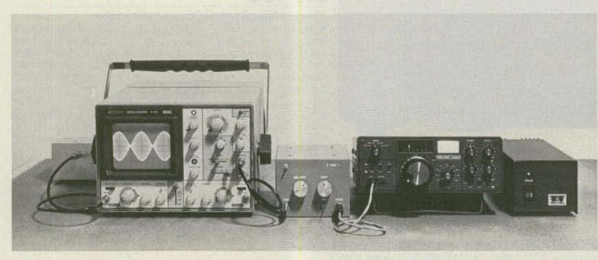
Photo B. Typical two-tone test setup. Refer to the text for high-power testing precautions. 36 73 for Radio Amateurs • April, 1985
