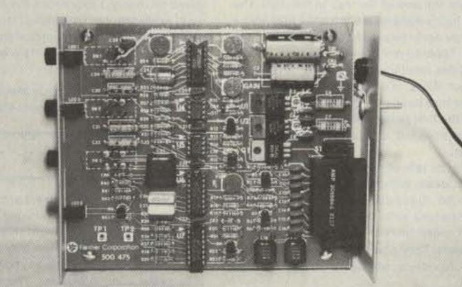
Photo B. The completed printed circuit board of the kit version.
