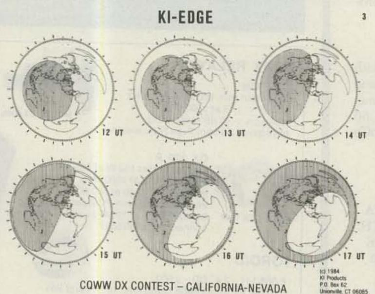
Fig. 1. The KI-Edge, terminator, or gray-line, indicator.
