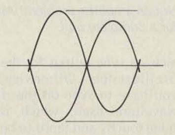
Fig. 2(e). Carrier leakage.
