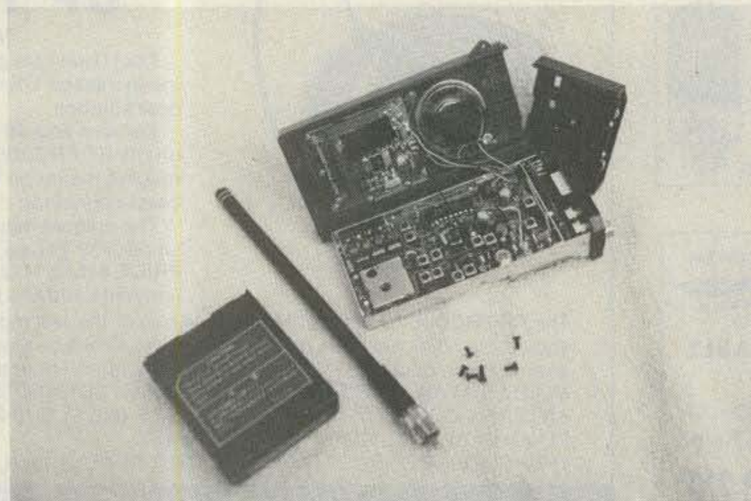
With its cover off, the TH-21A reveals a well laid out transceiver. On the left is the slide-on battery.
