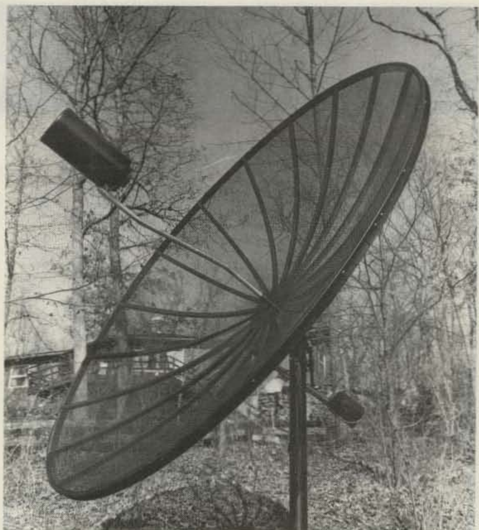
Ten-foot mesh dish from Kaul-Tronics.
