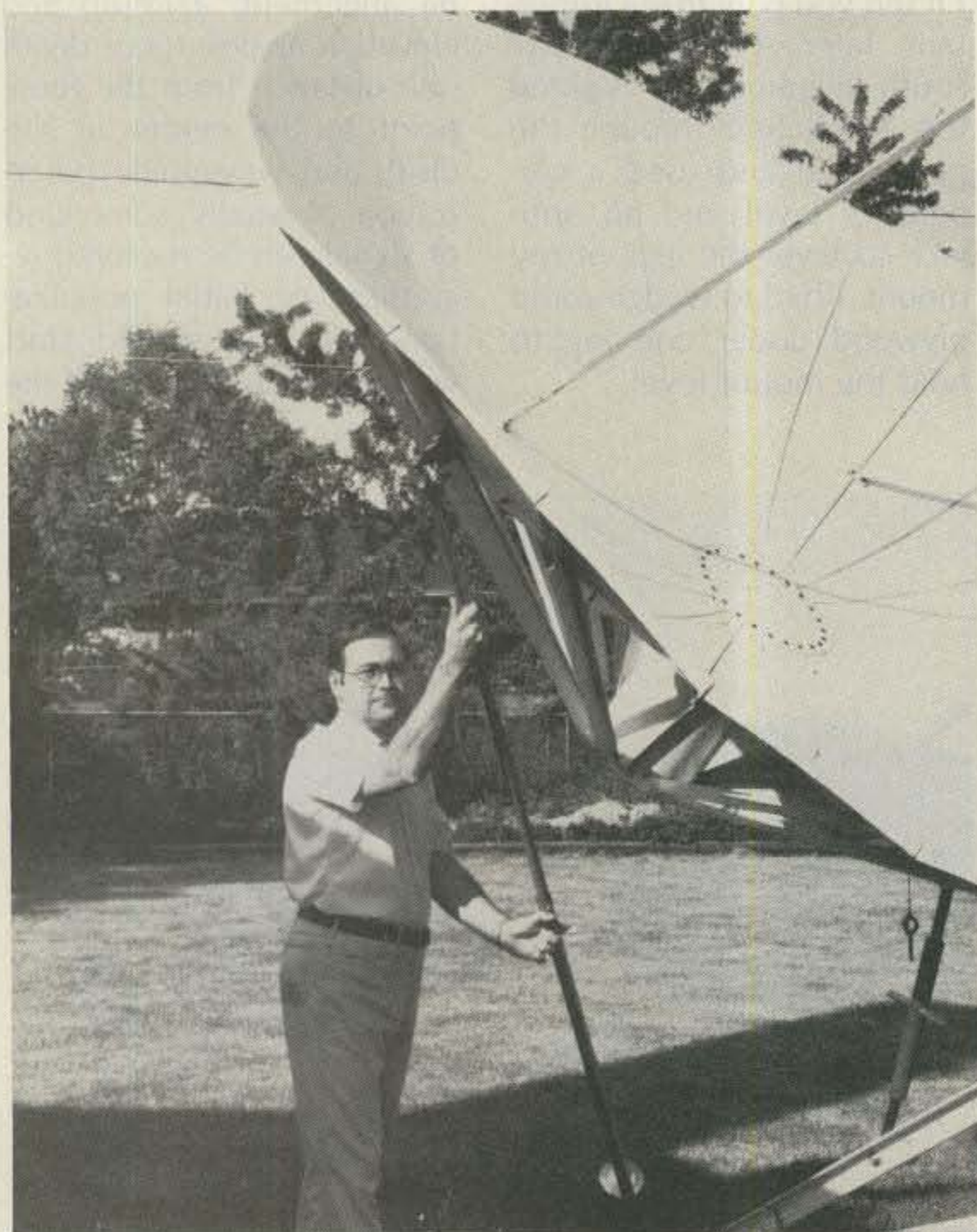
Photo E. To change satellite, just slide the telescoping tube a few inches and tighten the wing nut.
