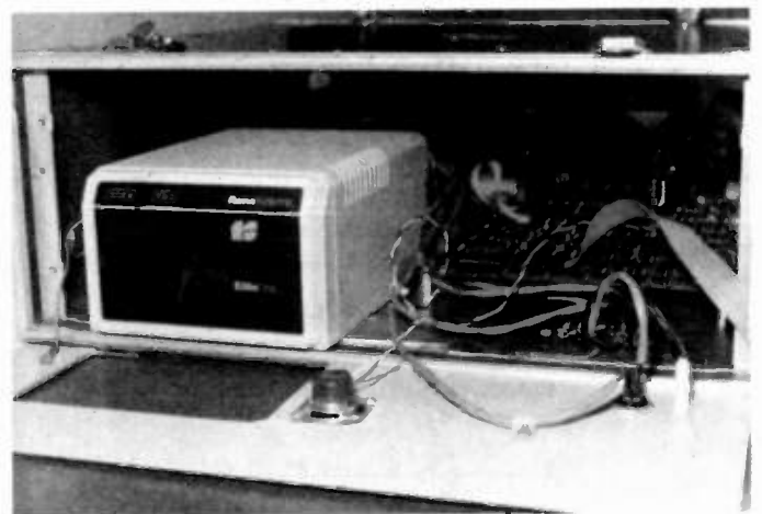
Photo B. Front of the case with the cover removed. Note the position of the disk drive and the motherboard. The terminal strip on the right is for distribution of the ac power. The copper-clad printed-circuit material can also be seen.
