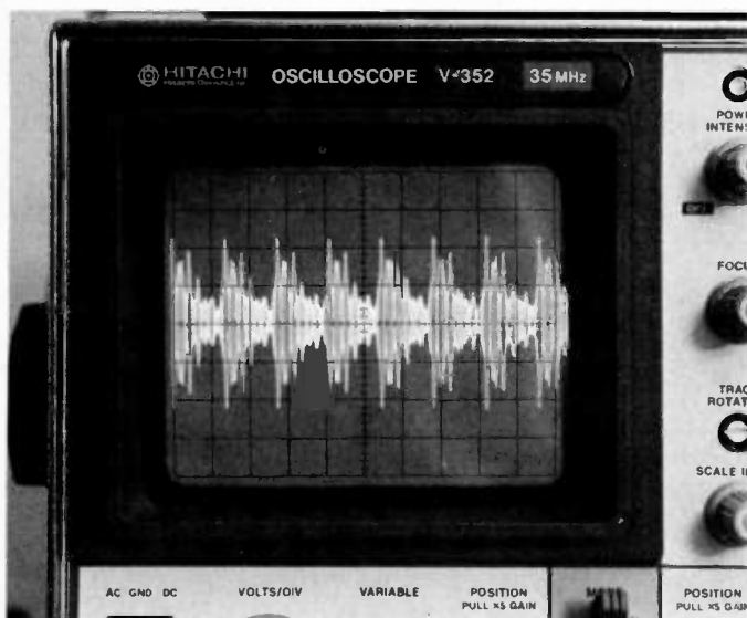
Photo B. Typical mini-ceiver SSB voice waveform. About 1.5-W p-p output.
