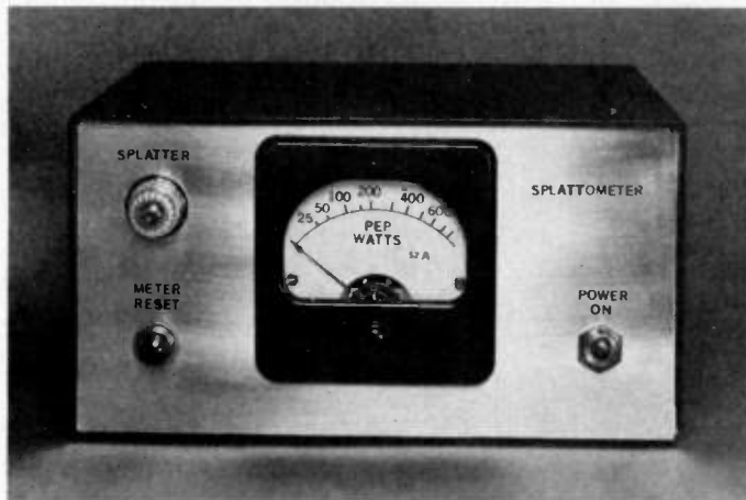
Photo A. The uncluttered 4" by 7½" front panel is dominated by the PEP wattmeter and splatter-alarm lamp. Only two operating controls are required, a power switch and reset push-button.
