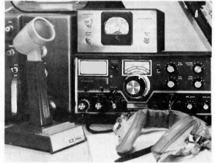
Photo D. Although it fits nicely on top of the transceiver, the Splattometer can be placed anywhere within the operator's field of view. It doesn't need constant attention; when you splatter, it lets you know with a bright flash.
