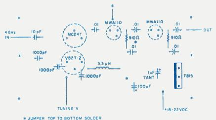
Fig. 4(b). Parts placement, foil side view.
