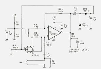
Fig. 1. Original circuit of the Amazing Audio Elixir (with correction).
