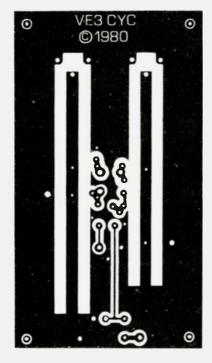
Fig. 11. One-stage preamp board PCB layout.
