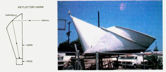
Fig. 4. The horn/reflector antenna is just a segment of a parabola fed by a very long horn. It has been in use for many years by A.T. & T. and other terrestrial microwave users. This design is considered by many as the ideal solution to high gain and low side-lobe response.
