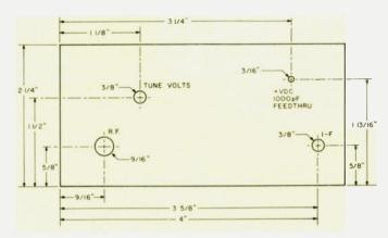
Fig. 3. Drilling template for 2" by 4" minibox.
