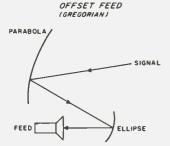
Fig. 5. The offset feed dish is similar to the Cassegrain in the two-reflector configuration, though single-reflector versions are also used. Sidelobe response is greatly improved because of a lack of aperture blockage.
