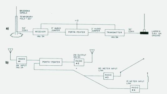
Fig. 5. Layout (a) shows a typical 2m hookup, and (b) a 3-band input command center. All inputs show up on 146.94 out. Mode has no effect on the system (i.e., CW, SSB, FM).
