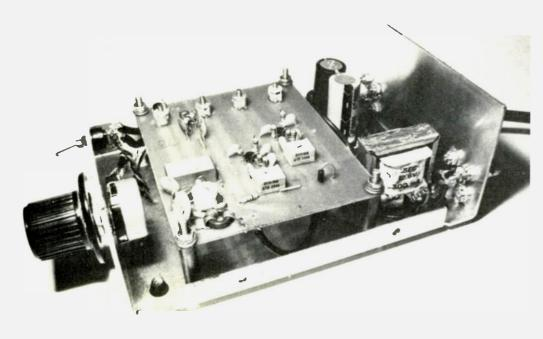
Photo B. Inside view of the converter showing PCB mounted on standoffs.
