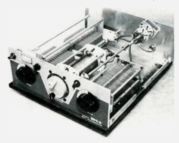
My home-built SPC transmatch uses the dual-section air-variable capacitor mentioned under the photo of the "junk." The single-section air-variable, the roller inductor with turns counter, and both vernier drives were salvaged from a junked military surplus transmitter purchased for \$12 at a hamfest. The transmatch cabinet was designed to blend with my Drake equipment.
