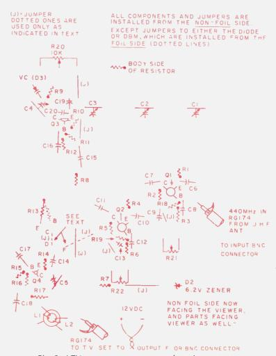
Fig. 8. ATV converter component location.
