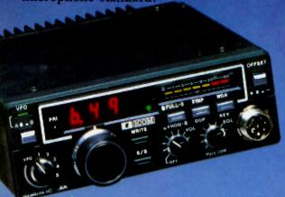
The best 2 meter multimode mobile on the market today, the IC-290A has features to make multimode mobile a snap. 2 VFO's, 5 memories, priority channel, memory and band scanning, squelch on SSB, selectable AGC and NB, and RIT. Touchtone ™ encoding provided with HM-8 microphone standard.
