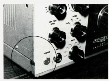
Don't let minor damage like chipped paint and superficial scratches (circled area) deter you from a good buy on an otherwise clean, operable rig.
