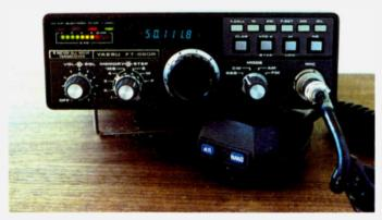
The Yaesu FT-680R six-meter transceiver. (Photo by KA1LR)
