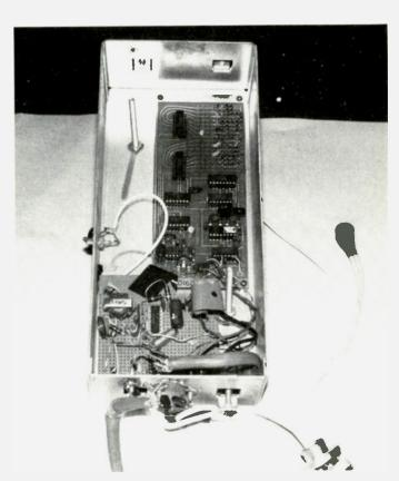
Photo B. Inside view of first unit from Photo A. CW IDer takes up most of box. Control system is in front.
