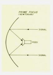
Fig. 1. The prime-focus design uses a parabolic reflector to concentrate the signal from the satellite into a small area known as the focus point. The accuracy of the dish surface to a true parabolic curve governs the size of the focus point and placement of the feedhorn.
