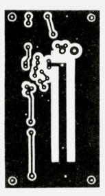
Fig. 9. UHF oscillator board PCB layout.
