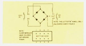
Fig. 2. Double-balanced mixer hookup details.
