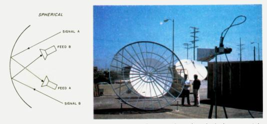
Fig. 3. Carve out a piece from a very large metal ball and you have the spherical antenna. It is possible to receive several satellites at once using separate feeds or you can simply mount the feed and LNA on a tripod and move it from satellite to satellite.
