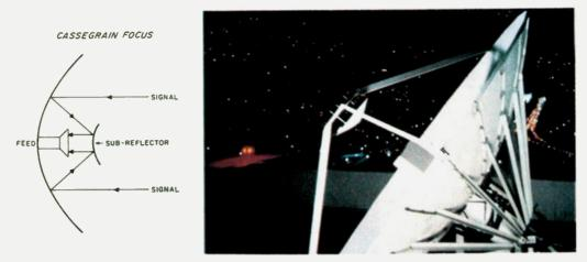
Fig. 2. The Cassegrain or twin-reflector design offers increased efficiency, but there are limits. As a rule, Cassegrains must be larger than ten feet before you can derive any benefit because the subreflector blocks a significant portion of the signal from ever reaching the dish.
