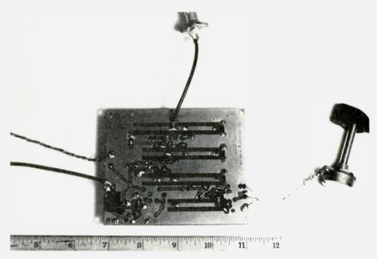
Photo C. Foil side view of converter with input, output, power, and frequency control connections.
