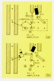
Fig. 4. Mixer installation details. (a) Double-balanced mixer. (b) UHF diode mixer.
