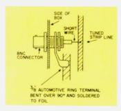
Fig. 5. BNC connector mounting.
