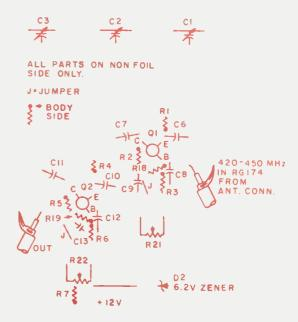
Fig. 14. Two-stage preamp board component location.
