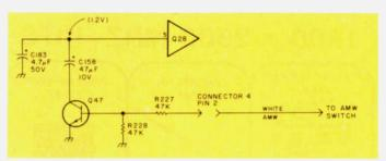
Fig. 2. Additional circuit on O28 shown in service manual. This extends low-frequency response on AM wide.
