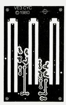
Fig. 13. Two-stage preamp board PCB layout.
