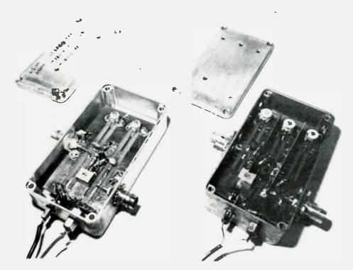
Photo D. Completed preamps in metal enclosures.
