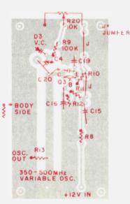
Fig. 10. UHF oscillator board component location.
