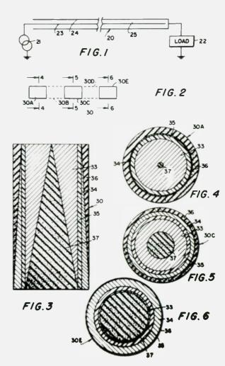
Fig. 6. Capacitance-compensated cable.
