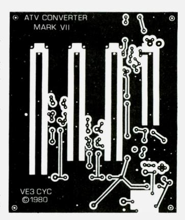
Fig. 7. ATV converter PCB layout.
