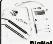
The Drake DM2350 Digital Multimeter is a convenient, small handheld liquid crystal display meter ideal for the serviceman or hobbyist. This 3½ digit meter is auto-ranging. auto-zeroing, has polarity indication, and an over-range warning signal. Battery life is greater than 300 hours with a "low battery indicator. A continuity test sounds a signal when circuit resistance is less than 20 ohms Dc accuracy is a basic 0.8%
