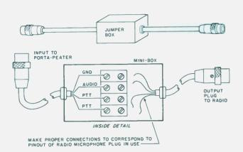
Fig. 6. A jumper box will solve the problem of a fistful of audio cables. Use shielded box and cables only.
