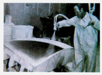
Fig. 6. Nearly ideal reflector surfaces are possible when flame-spraying is applied to fiberglass dishes. Care must be used in the coating as well as curing time for the resin to ensure that the dish will follow the proper curve within 1/8 inch.
