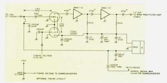
Fig. 1. Satellite downconverter schematic. \*=chip or disc ceramic.
