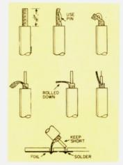
Fig. 3. RG-174 coax preparation and installation.
