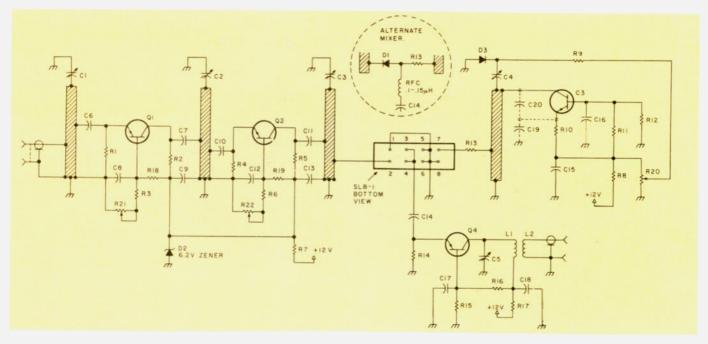
Fig. 1. ATV converter schematic.
