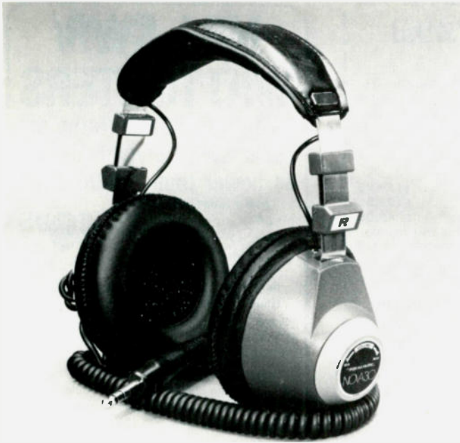
A good pair of headphones will last a lifetime of hamming. Though communications-type phones are usually recommended, high-quality stereo headphones are often preferred because they usually sport extra-soft, oversize cushions and padded, adjustable headbands. An adapter cord or plug would be required to convert a stereo phone such as this Radio Shack unit for monophonic use with your receiver or transceiver. (Photo courtesy of Radio Shack)
