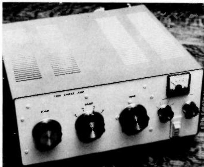
Photo A. Front view of amplifier showing all controls and taped top louvers.
