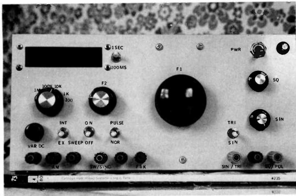
Photo A. The completed swept function generator. The knob labeled F1 is the primary frequency control and is mounted on a 3:1 gear drive. The SIN/TRI output jack also provides a ramp function. All unlabeled jacks are grounds, except the jack, far left, which is the variable dc output.
