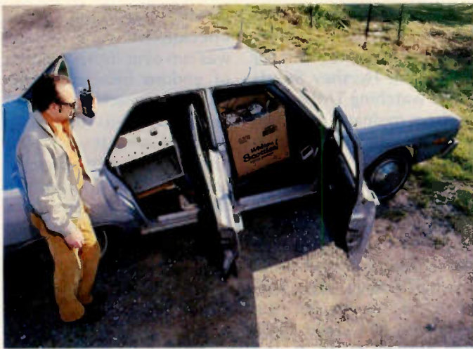
Frank N3RZ stands next to his portable repeater, a .70/.30 220 repeater linked to the main .40/.64 machine to extend coverage. The duplexer is in front seat, the machine and battery in the back, and the antenna is on the car roof.
