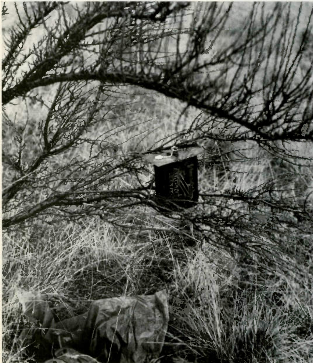
Photo A. The jamming transmitter in the sagebrush, enclosed in a black-painted first-aid box. Wires lead to the plastic-wrapped, buried batteries.
