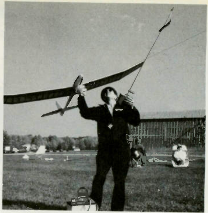
Don Goodwin WA2FRO puts his 100-inch-span Aquila on the tow line. The plane carries a Thermic Sniffler and is guided by an R/C rig on 53.3 MHz.
