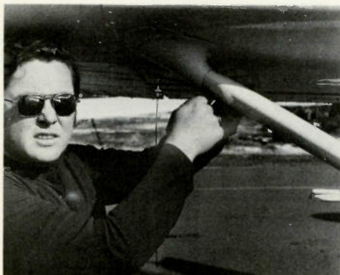
Photo A. Connecting the antenna onto the mount and running the coaxial cable down the trailing edge of the strut.
