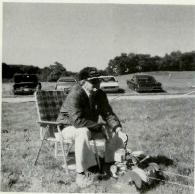
Joe Bertin WD8PRG operates a winch-line retrieval system which returns the towline to the launch area for another launch.
