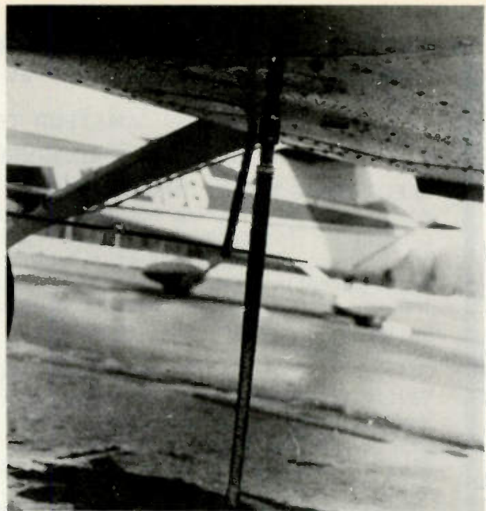
Photo F. The inspection plate mounted on the belly with a 10-meter band rubber duckie antenna attached.
