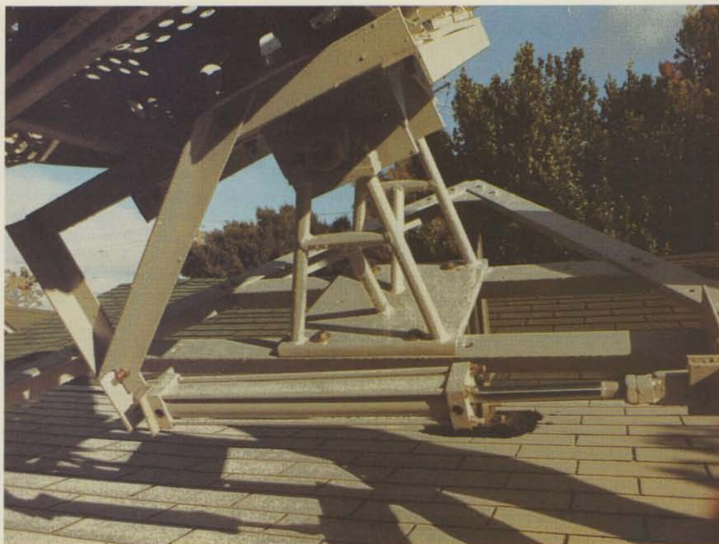
Photo B. Close up of the azimuth steering arm and control cylinder.
