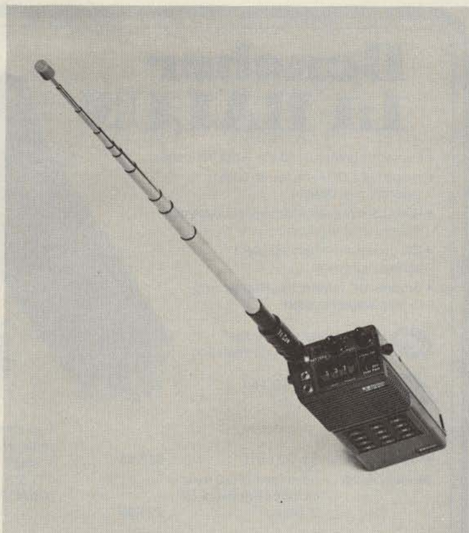
Partially extended VoCom 5/8-wave 2-meter HT antenna is shown here installed atop an Icom IC-2AT transceiver. Tension antenna is base-matched and boasts a 5.6-dB gain over a 1/4-wavelength whip and as much as a 10-dB improvement over stock rubber ducky antennas, according to the manufacturer's measurements. (Photo courtesy of VoCom Products Corp.)
