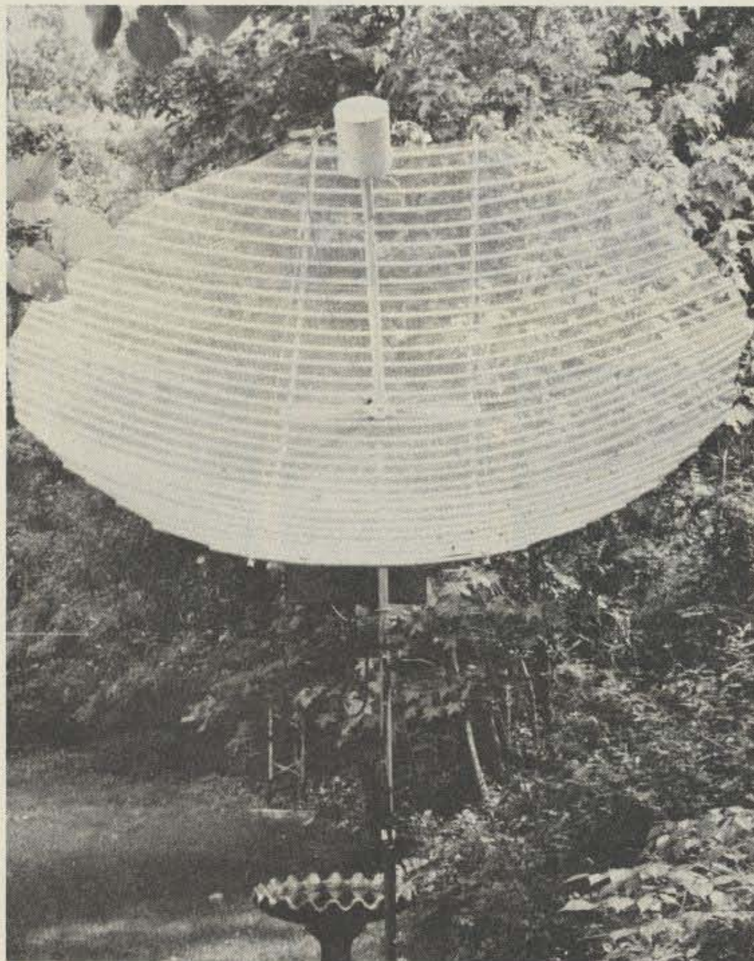
Photo A. 8-ft. parabolic reflector. Elements are 5/8" aluminum tubing spaced 3". Reflective surface is reinforced with ¼" hardware cloth. The cylindrical horn is a 2-lb. coffee can with probe.
